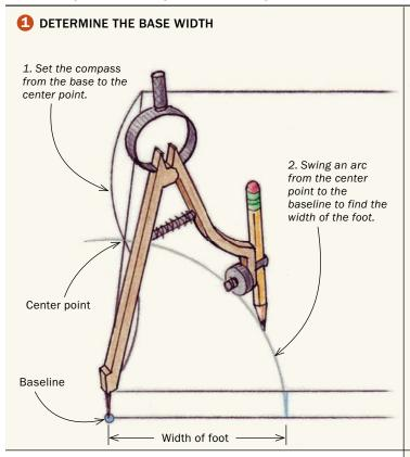
Start with the width. Set the compass equal to the distance from the outside corner of the base of the foot to the center point of the diagonal you drew earlier. Swing an arc from the corner down to the baseline. This defines the width of the foot. From this point, draw a square line up to the top of the foot.
