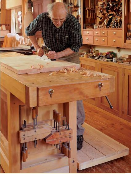
**More height means more power.** The platform allows Becksvoort to work at a height that's most effective and ergonomic for planing a wide panel.
