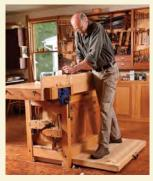
Standard workbench height is great for most hand- and powertool tasks, but sometimes it pays to gain a higher stance or to elevate the workpiece.
