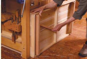
**Tucked away until you need it.** Becksvoort built a platform to store perfectly between the legs of his bench. Limited by the clearance beneath the bottom rail of the bench, Becksvoort added a lift system under the platform. Once he pulls the platform out, he can add to its height by folding down hinged risers.
