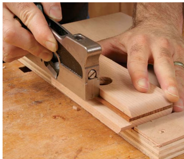
Keep the skate running smoothly. Use a shoulder plane to take a few light shavings off the skate, and don't forget to wax the skate before use.
