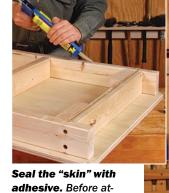
adhesive. Before attaching the base top and bottom, apply a thin bead of construction adhesive to the frame. Nail on the plywood "skins" with 2-in. ribbed nails, spacing them about 4 in. apart.
