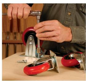
Attach the casters. White uses 1½-in. lag screws to attach the casters securely to the base. Typically, the corner blocks will support lag screws for only three of each caster's mounting holes, but that's enough.
