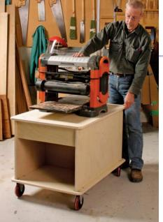
Use this cabinet-style base for bench-mounted tools, such as thickness planers, drill presses, and miter saws. It's made entirely of Baltic-birch plywood. This 26-in. by 40-in. base is sufficient for most benchtop tools. Once again, modify measurements to suit the size of the base you need.
