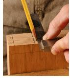
Mark the widths of the tails on the end. Set the pencil point into the depressions from the points of the dividers, slide a square up to the pencil point, and draw lines across.
