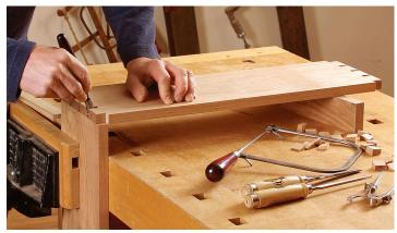
**Use the tail board to mark out the pins.** Line up the baseline of the tail board with the inside edge of the pin board. Now use a marking knife to transfer the tail locations clearly to the pin board.
