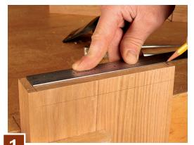
**Mark the pin width.** Stack both tail boards in the vise. After laying out half-pins, mark the pin width on one end.
