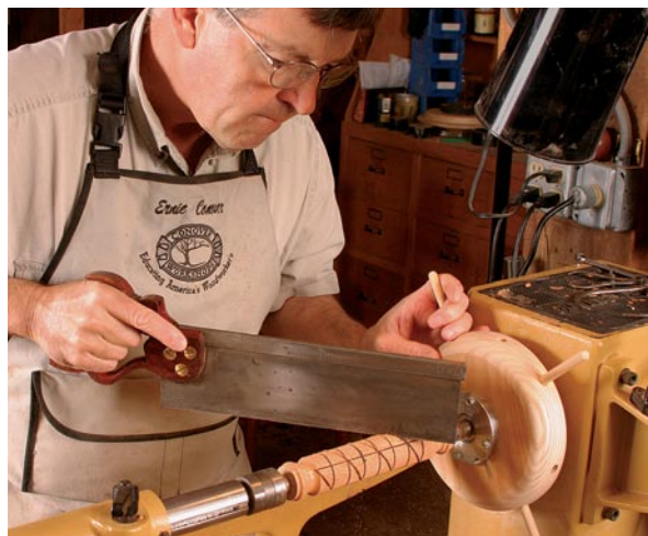
Saw the layout line. Use a backsaw to cut a kerf roughly \frac{1}{4} in. deep along the spiral lines. Gradually spin the piece by hand as you cut.
