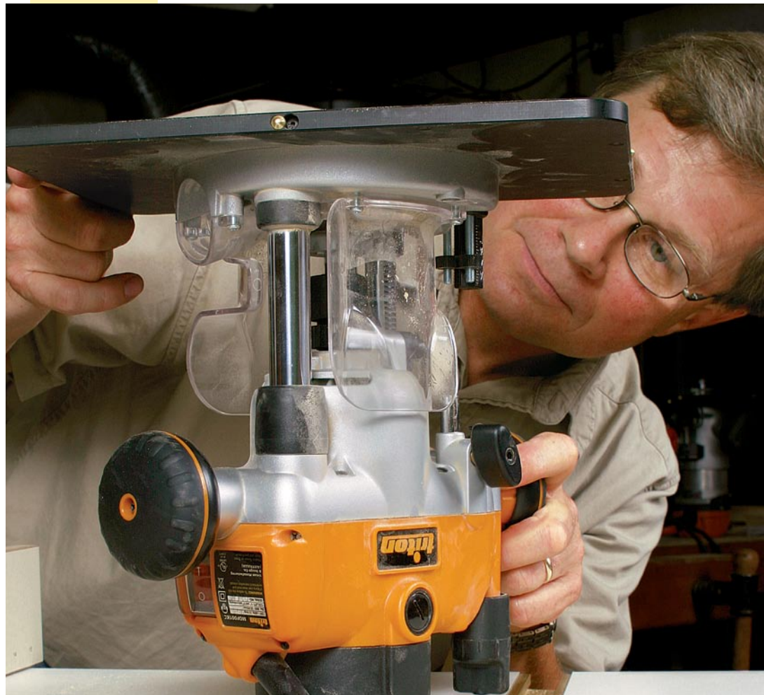
Dust collection. A plastic shroud around the Triton's base does a good job of directing dust to a shop-vac hose. None of the other routers has a good dust-collection design.
