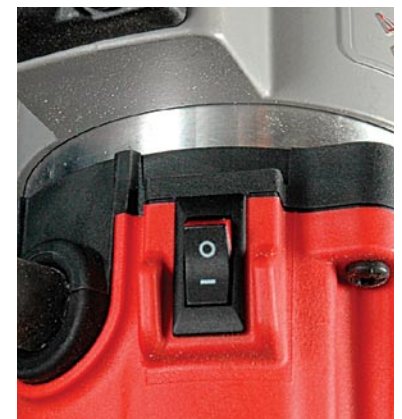
Switch styles. The Freud's large slide switch (left) is slightly easier to reach and use than a small rocker switch such as the one on the Milwaukee (above).
