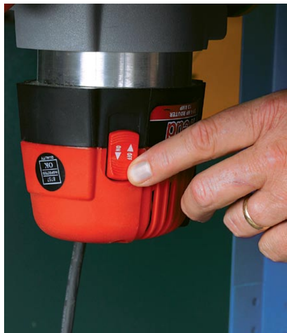
Switch styles. The Freud's large slide switch (left) is slightly easier to reach and use than a small rocker switch such as the one on the Milwaukee (above).
