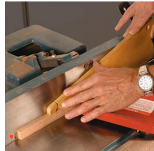
2 Joint two faces. These will serve as reference surfaces for final trimming of the runners to fit in the miter-gauge slots.
