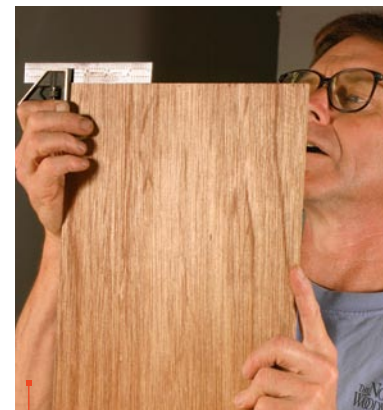
3 Check the cut with a square. Any gaps will help you determine the direction and amount of adjustment the fence requires.
