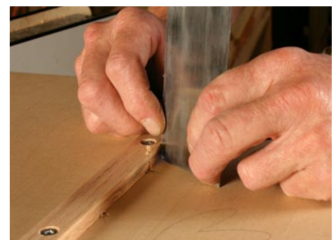
5 Trim the high spots. Push the completed sled back and forth in the slots a few times. Any places where the runners rub against the side of the slots will darken. Trim these areas with a scraper, then wax the runners and the bottom of the sled to reduce friction.
