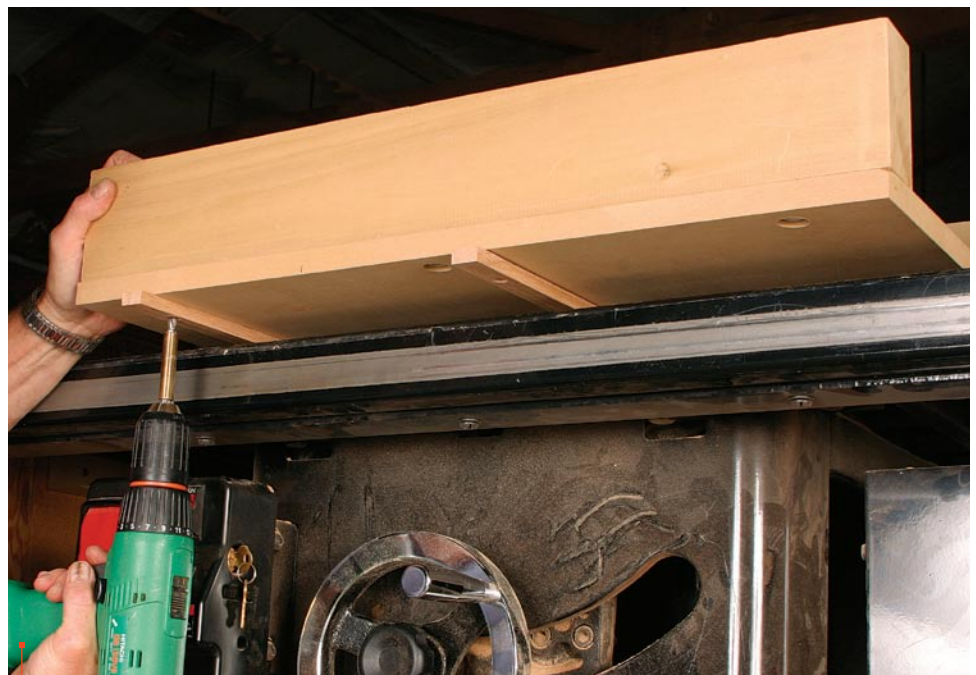
4 Attach the runners. Assembling the sled with the runners in their slots helps ensure they'll be parallel and properly spaced when you're done. Attach the runners with wood screws driven into countersunk holes.
