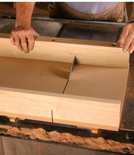
1 Make the kerf. Set the blade to its full height and cut through the sled.
