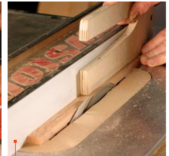
3 Trim to final width. Take light cuts and check the fit in the slot as you go. You also can use a planer or a handplane.
