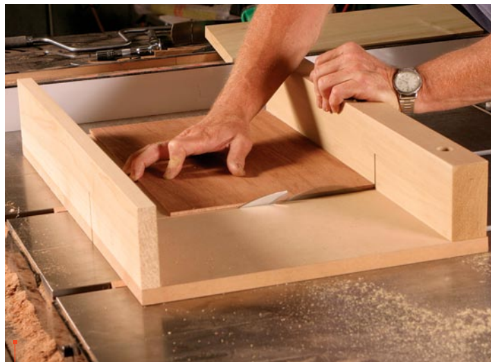
2 Make a test cut. Crosscut a piece of wide stock to gauge the fence's accuracy.
