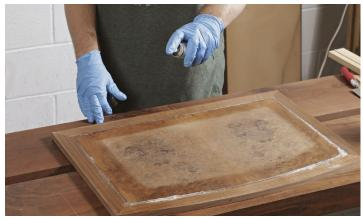
**Speed up the drying.** Holding the can about 12 in. above the table, spray accelerator over the glue to set it immediately.
