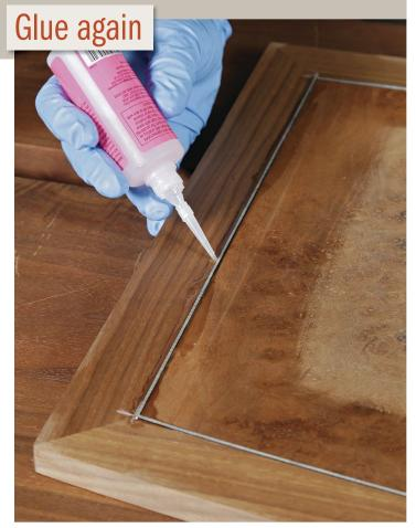
**Flood the surface with glue.** Complete the glue-in by flooding the surface with a thin cyanoacrylate glue. A thin-tip nozzle keeps the glue on top of and immediately next to the inlay.
