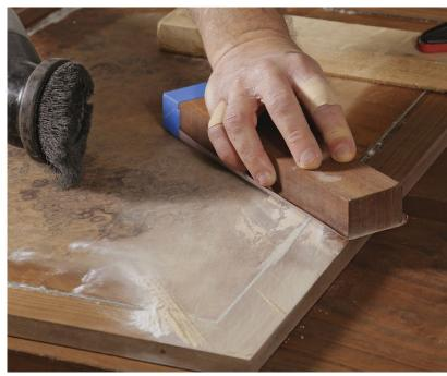
**Sand the inlay flush.** Wrap blue tape several times around one end of the sanding block (top). This raises the taped end off the surface and focuses the sanding on the inlay, keeping the sandpaper off areas that don't need sanding. Thibodeau uses a vacuum hose to collect dust as he sands the inlay level with the top (above).
