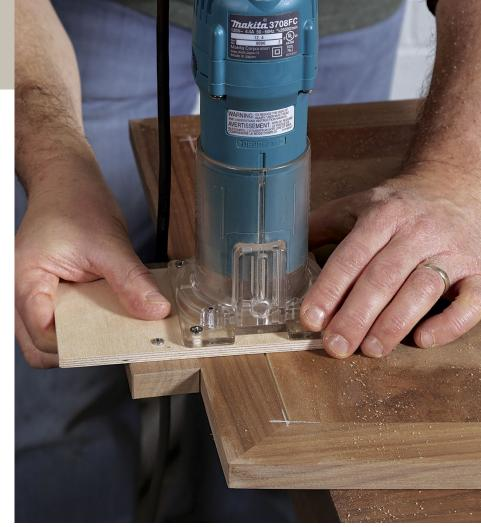
**Fence keeps the bit on course.** A short, straight piece of hardwood screwed to a long base ensures that the groove is parallel to the edge.
