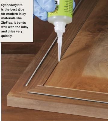
**Glue goes in the groove.** Use a medium thickness cyanoacrylate glue. A needle tip on the bottle gets the glue into the groove without getting it on the table's surface.
