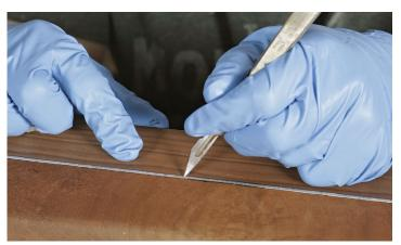
**Seat unruly inlay.** Should the inlay rise up, press it back down with the point of an X-Acto blade. The cut made by the knife is so fine that it doesn't show up after a finish is applied.
