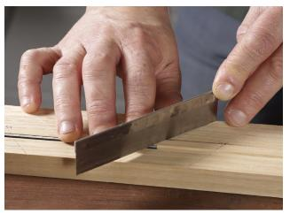
Cut miters with a model-maker's saw. A guide kerf in the fence against which the inlay is held ensures an accurate cut.
