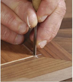
**Square the corners.** Thibodeau uses a shopmade chisel (see p. 24) with a profile that's thin enough not to damage the wall opposite the one being pared.
