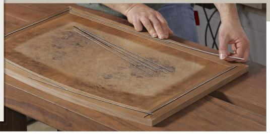
Lay out for length. Before cutting the inlay to length, place pieces beside the grooves, overlapping the ends, to get a sense of how much inlay is needed and where joints will fall.
