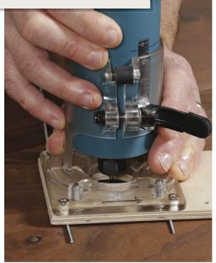
**Set the bit's cut depth.** After placing the router on two pieces of inlay, lower the bit until it is just shy (0.005 in. to 0.010 in.) of the benchtop.
