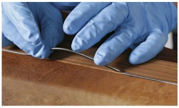
**Flex the last piece.** Butt the end of the last piece against the end of the adjoining piece, and then press down on the inlay. This technique pushes the two ends together tightly, making for a gap-free joint between them.
