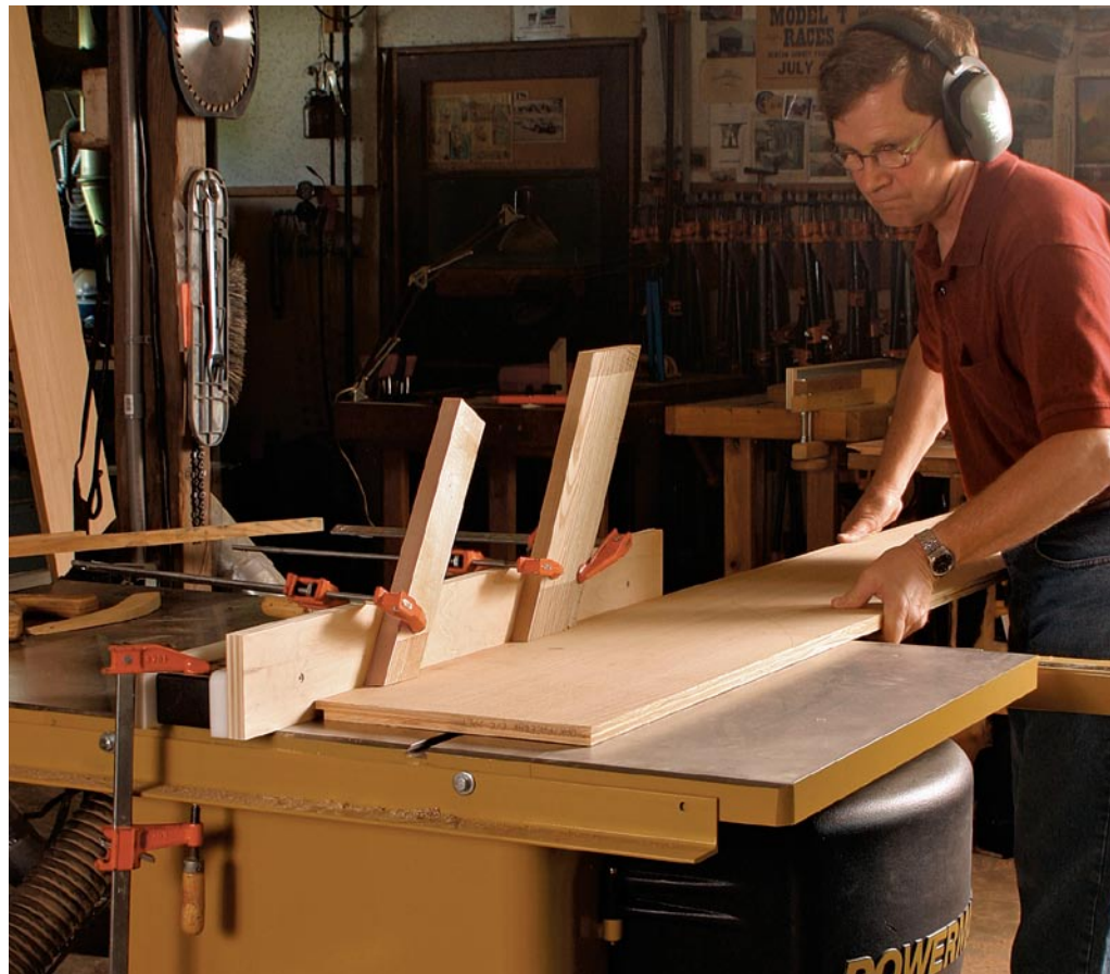
Fence-mounted featherboards apply pressure from the top down. This keeps stock firmly against the table for tasks like rabbeting an edge on the tablesaw (right) or cutting a molding profile or edge treatment on the router table (above).
