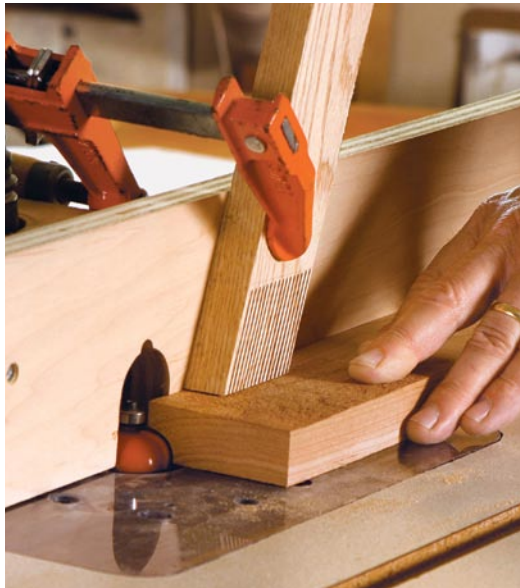
Fence-mounted featherboards apply pressure from the top down. This keeps stock firmly against the table for tasks like rabbeting an edge on the tablesaw (right) or cutting a molding profile or edge treatment on the router table (above).
