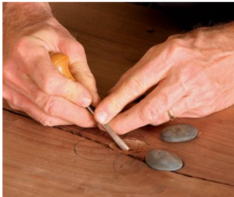
Remove the waste stock. A carving gouge pares stock as needed so that each stone can be inlaid to about one-half its thickness.
