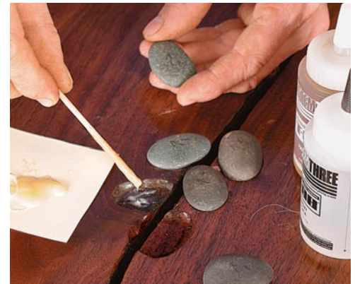
Glue the stones in place. A two-part epoxy bonds the stones securely to the top. Stones that span the gap are glued to one side only.
