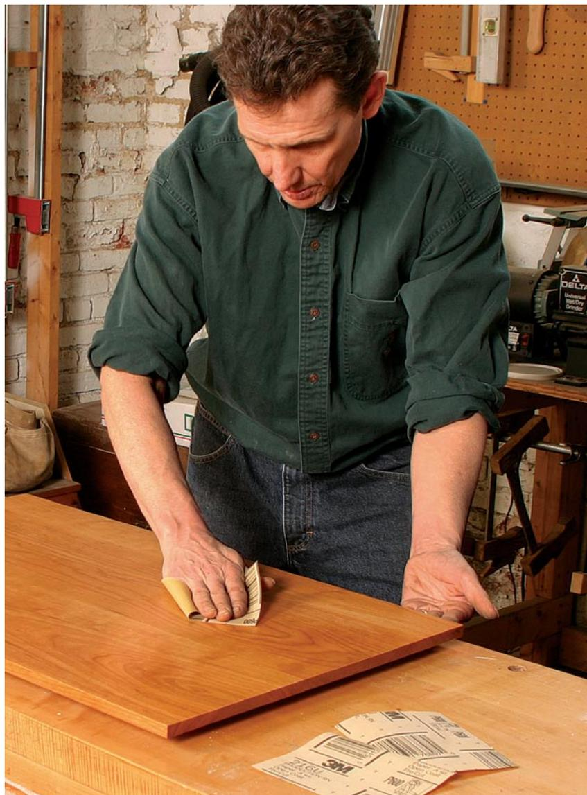
or debris can be rubbed out with some 600-grit (CAMI grade) sandpaper followed by 0000 steel wool after the shellac has cured for about eight hours. Because there are no “coats” of finish in the conventional sense, just keep applying the finish to achieve the look you want.
