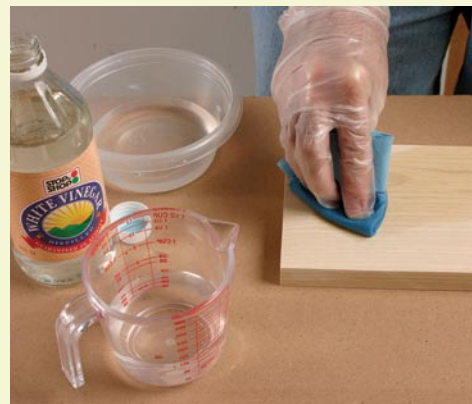
Neutralize the bleach. When the wood is the desired lightness, apply a mixture of white vinegar and water to stop the chemical reaction.
