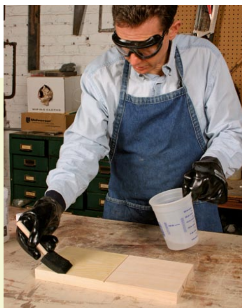
Brush on the bleach. Combine the two bleach components in a nonmetallic container and apply the mixture to the wood.
