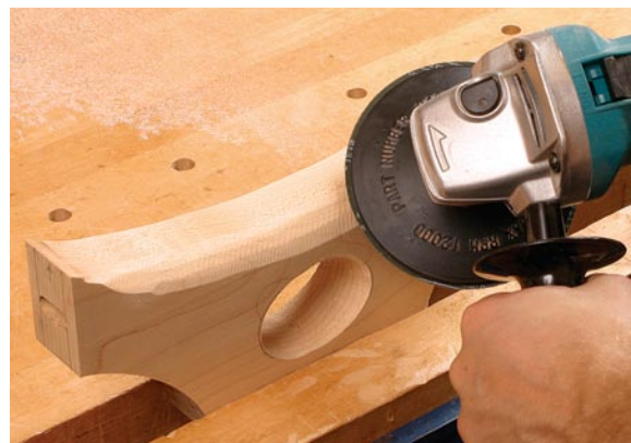
Some grinding is best done before assembly. Some areas will be easier to reach now. To ensure symmetry and flowing joints, leave the bulk of the grinding for afterward.
