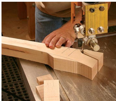
After mortising, rough out the curves. Cut right to the layout lines; these bandsawn surfaces will guide the shaping process later.
