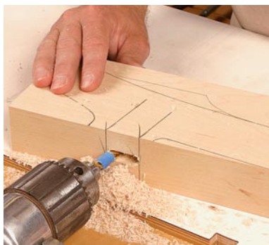
A simple setup for angled mortises. Williams uses a simple shopmade horizontal mortising table, moving the heavy workpieces by hand as he eyeballs the layout lines.
