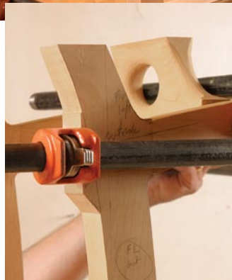
Clamping requires square surfaces. Note the stock left in strategic areas to serve as clamping pads. Be sure each joint closes completely.
