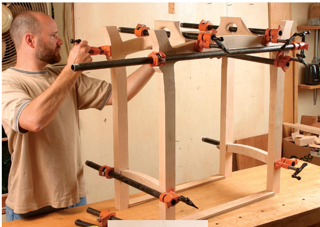
Clamping requires square surfaces. Note the stock left in strategic areas to serve as clamping pads. Be sure each joint closes completely.
