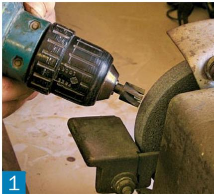
**1** **Modify a plug cutter.** Chucked in a variable-speed drill, the cutter is slowly rotated into a spinning grinding wheel. Dip the cutter frequently in water. When done, grind a slight back bevel on the tip of each tooth.
