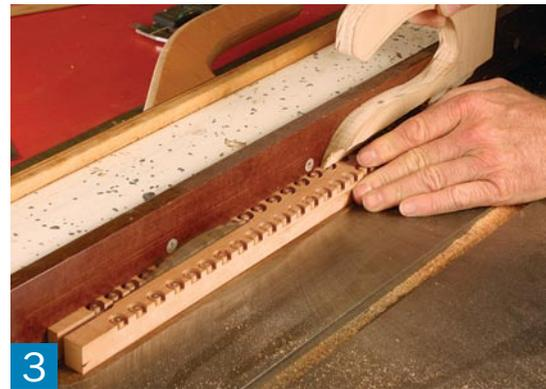
**3** **Rip strips to form the pegs.** Keep the stems centered on the pegs as you create the desired peg width (in this case, a 5/16-in. square needed a cut 1/2 in. to either side of the 1/4-in.-dia. stem).
