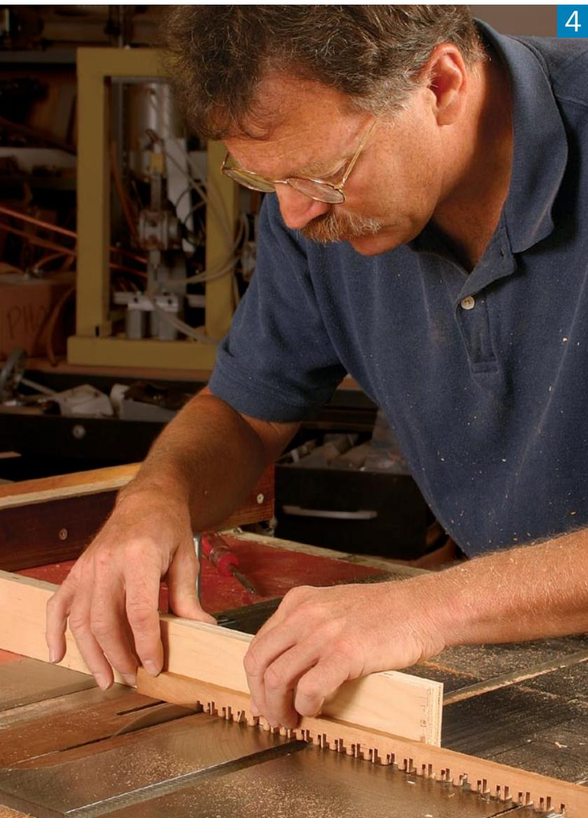
**4** **Crosscut the pegs.** A shopmade indexing jig allows you to register one side of each stem against a brad so that the saw cuts the side of the cap exactly 1/32 in. away from the stem. After completing all of the cuts on one side of the stems, turn the piece around and cut the other side.
