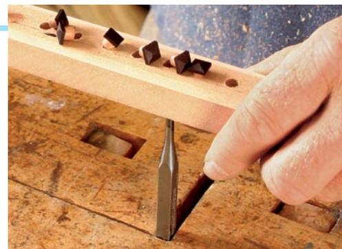
**Remove the pegs.** Use a rod or nail punch, clamped in a vise, to press each peg out of the jig.
