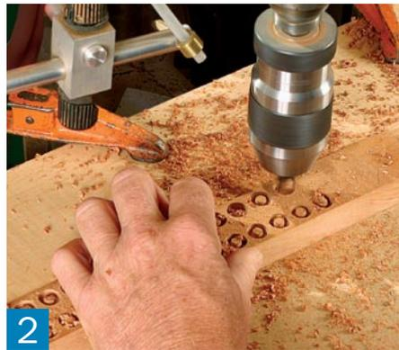
**2** **Drill the stems with the modified cutter.** The distances between the stems are not important, but use the depth stop on the drill press to keep the lengths of the stems consistent and clamp a fence to the drill-press table to keep the rows straight.
