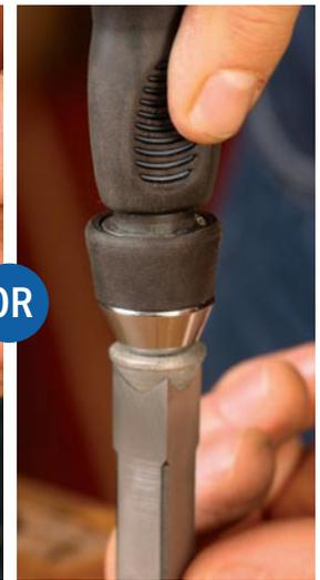
**Hone the bevels.** A little work with a round slip stone (left) or a special, cone-shaped, diamond-coated abrasive (right) produces fresh, sharp edges that ensure a cleaner cut. Use a flat slip stone to remove the burr that results.
