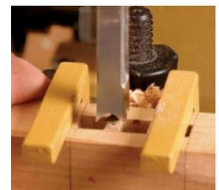
*Make two cuts, one at each end of the mortise (left). Then make a series of cuts, leaving a web of wood in between each cut. Last, make cuts (above) to clean out the webs.*
