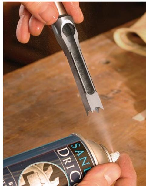
**Add some lubricant.** To help reduce friction during cuts, spray both the chisel and bit with dry lubricant after sharpening. Later on, when cutting mortises, an occasional squirt of lubricant on the chisel and bit will fight friction.
