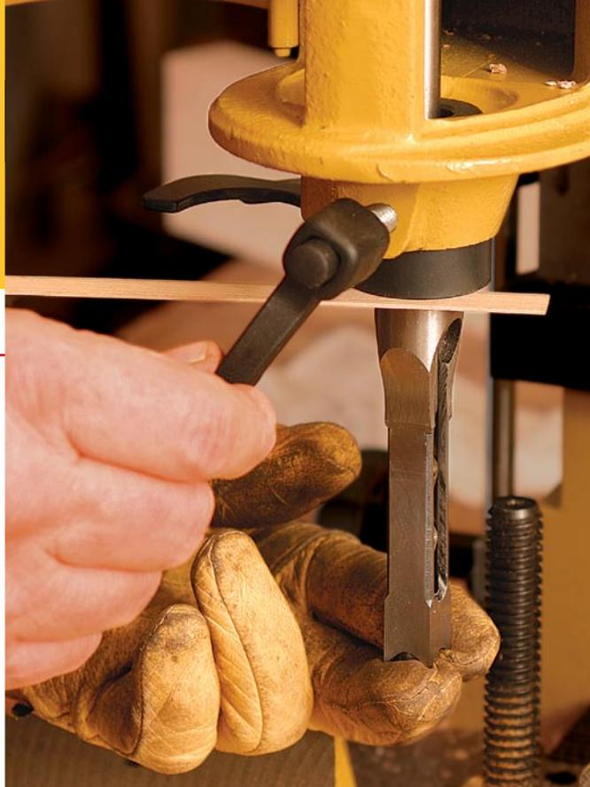
you need to sharpen. If the bit has a brad point, I usually sharpen the point, too. The machining process at the factory sometimes leaves ridges or burrs at the transition area between the spurs and flutes. Use a slip stone to smooth any you find. After that, polish the flutes with a medium-grit abrasive pad to create a slick route for the chips to follow.
