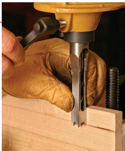
Remove the spacer and raise the chisel until it butts against the bushing. A squaring board ensures that the chisel is square to the fence. Tighten the locking knob.
