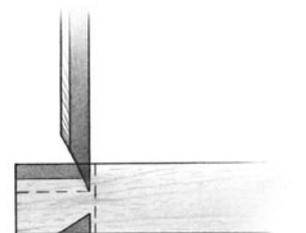
3. Finish by paring the tails to the scribed line and to the saw lines, working inward from both sides.
