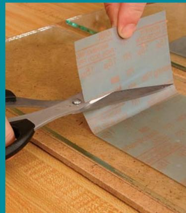
When a section of paper finally wears out, simply peel up the worn section and cut it off with scissors. Any residue from the adhesive backing can be removed from the glass using baby oil or mineral oil and a soft cloth.
