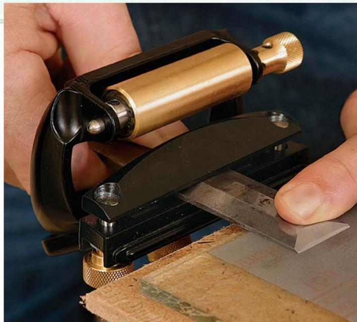
**Remove the burr on the back.** To remove the burr that forms on the back of the bevel edge, the final step is to place the back of the chisel on the 0.3-micron paper and slide it back and forth until the burr breaks off.
