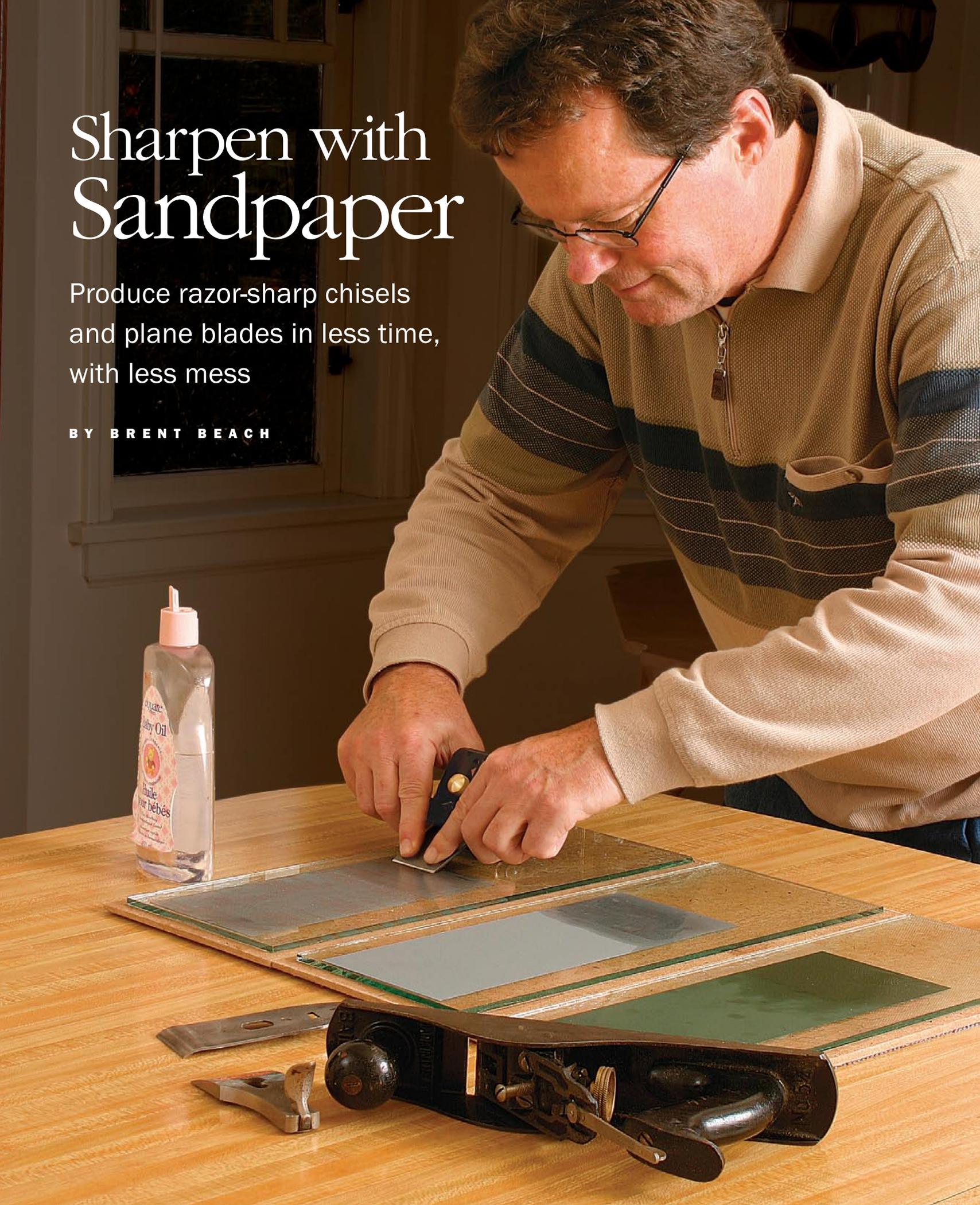
For years, no matter what method I used, my sharpening efforts were a disappointment. Then I tried high-quality sandpaper as the sharpening medium, used with an angle jig. To my surprise and delight, the process proved to be remarkably quick, easy, and effective. Indeed, it now takes less than two minutes on average to sharpen a dull plane blade or bench chisel with a perfect bevel angle every time.
