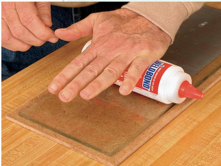
**Roll out the bubbles.** Air bubbles trapped under the paper can cause it to rip when sharpening. Use a roller of some sort to push the bubbles out to the edge.
