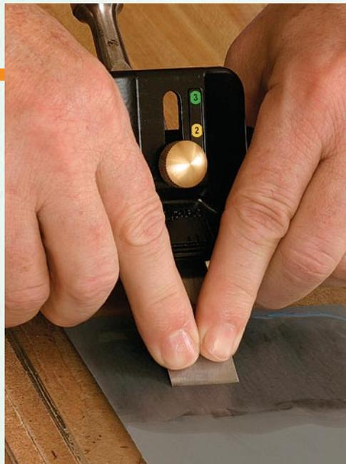
**Continue through the grits.** With the jig set to 31°, Beach hones the second microbevel on the 5-micron paper. He then raises the angle to 32° for the final passes on the 0.3-micron paper.
