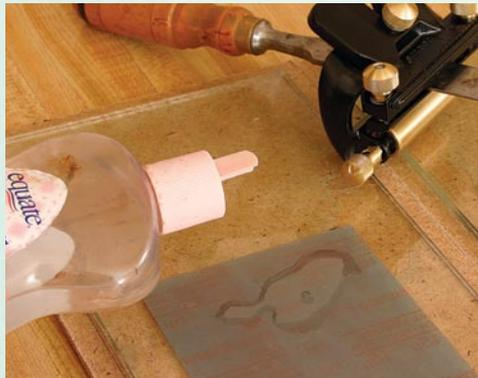
**Start with 15-micron paper.** Add a little baby oil or mineral oil to help float away the steel filings. Set the jig at 30° and roll it back and forth, keeping the wheel off the sandpaper. It takes a minute or less to establish the first microbevel.
