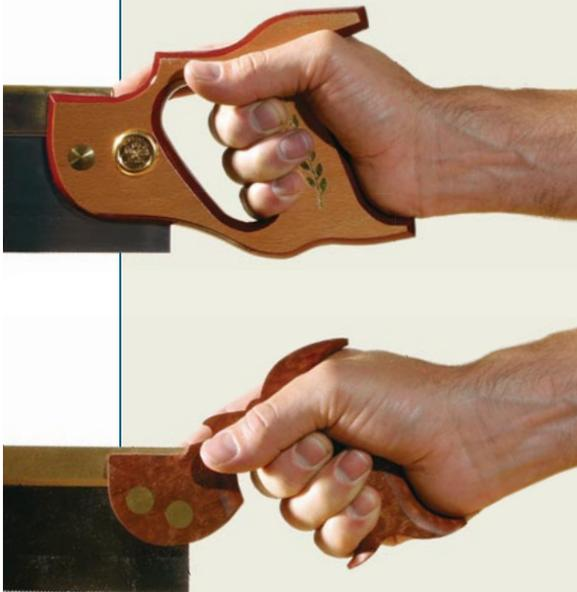
When considering a pistol-grip saw, be sure the angle between the handle and the sawblade (called the hang) is comfortable. Ultimately, the mounting angle will dictate how you hold the saw.
