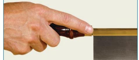
The turned handle of a gent's saw is designed to be grasped in the palm of the hand, with the index finger providing control.
