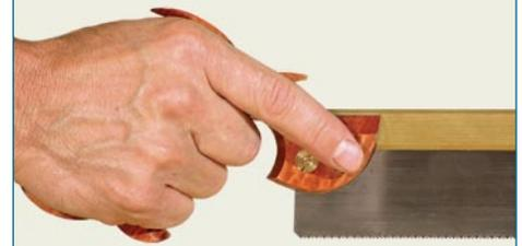
For comfort, use a three-fingered grasp on a pistol-grip saw, with the index finger pointing forward.
