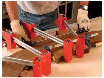
**Can you have too many clamps?** Blocks held to the segments with the red clamps provide purchase for small bar clamps to pull the segments together.
