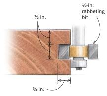
**Clearance for the last board.** The shorter boards slide into the groove, but the last one must be dropped into place. Working on the bottom of the ring, a flush-trimming bit removes the necessary material.
