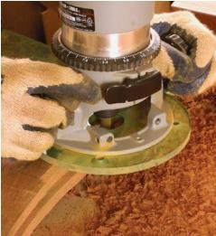
**Groove the ring for the top boards.** A ½-in. bearing-guided rabbeting bit makes the cut. To control the depth on multiple passes, successively smaller guide bearings are used until the groove reaches ¾ in. deep.
