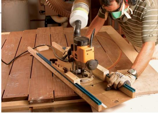
**Rout the tenons first.** To minimize tearout, the author uses a ½-in. spiral up-cutting bit and ¼-in. MDF spacers between the boards where the router will pass. Take shallow passes until the tenon thickness matches the groove in the ring.
