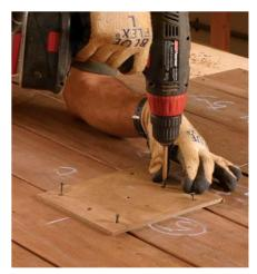
**Pivot block prevents marring the top boards.** Drive screws between the top boards to hold the block in place. A pivot pin in the trammel engages the center hole in the block.
