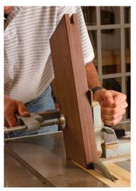
**Tenoning jig and a dado blade slot the segments.** Splines sawn from ipé scraps fit in the slots to secure the joints.
