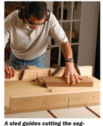
**ments to length.** Wedges cut to the 15° miter angle position the stock for crosscutting. The last two pieces won't be cut until the others are glued up, to allow for tweaking the final fit.
