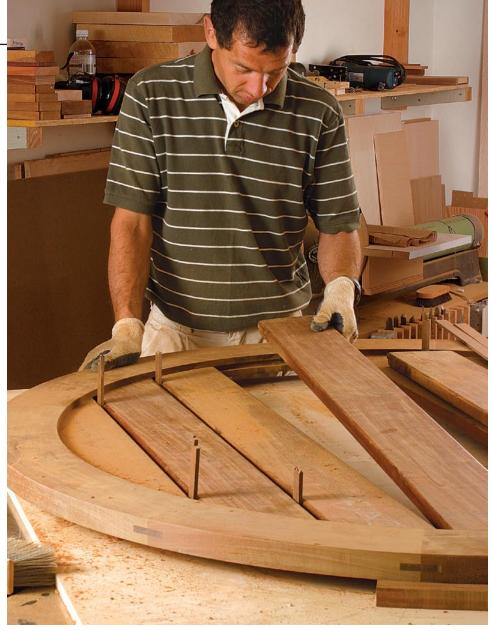
**Rabbeted top boards fit the ring.** Working from below, the boards are spaced with ¼-in. shims. A deadblow hammer adjusts them so that the final, center board aligns with the clearance slot.
