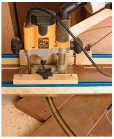
Adjust the trammel and rout the tenons to length. Cut a deep groove ¾ in. out from the tenon shoulder, stopping short of routing all the way through the boards. Unscrew the boards and finish the cut on the bandsaw.
