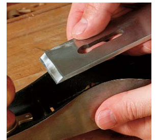
This side up. On a block-style plane, the bevel of the blade faces up.
