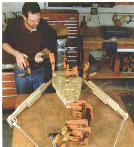
Clamps ease the bend. As the bend progresses, clamps help pull up the blank. Once the bend is complete, the assembly stays on the bending form for only a few minutes.
