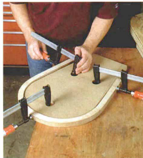
Cooling forms save space. Once the bend is complete, a cooling form, made of MDF, is a good way to store the piece for cooling overnight. Using cooling forms also enables you to bend other blanks almost immediately.
