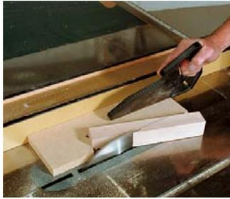
**Safer and simpler cutting with a jig.** The tablesaw jig ensures a straight, flat 20° taper-cut on the base of the plane, which is held in place by a screw.
