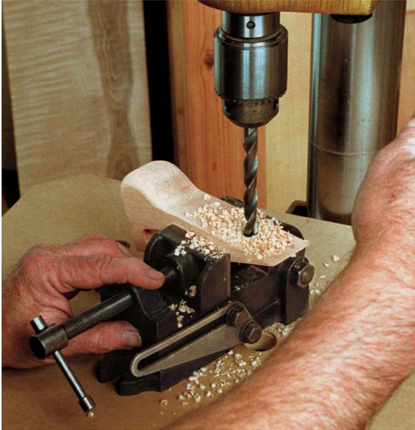
**Bore the hole for the threaded insert.** The hole is drilled at a right angle to the tapered portion of the base. Use a vise and square to position the stock for drilling.
