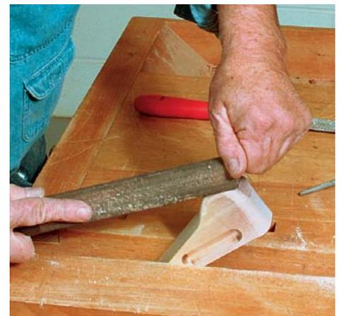
**Hand-shape the heel.** After bandsawing the rough shape, a few minutes with a rasp and file complete the rounding of the heel. Smooth out the file marks with sandpaper.
