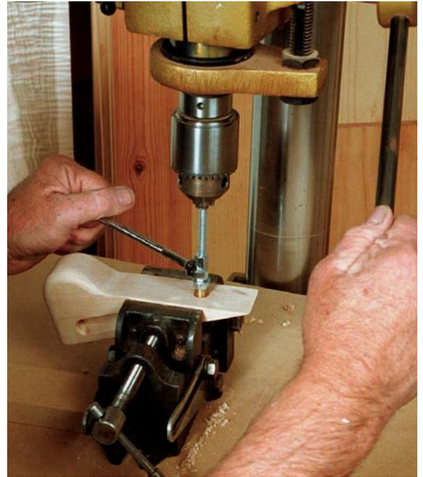
**Install the insert.** With the drill turned off, and with the help of a couple nuts, a threaded rod and a wrench, the insert goes in easier and straighter.
