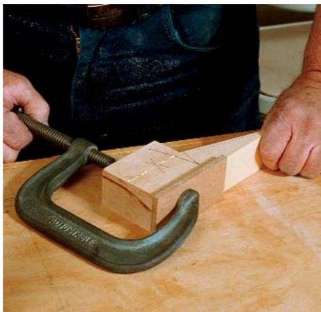
**Glue the heel onto the base.** The grain at the joint line matches nearly perfectly because the two parts are ripped from the same piece of stock.
