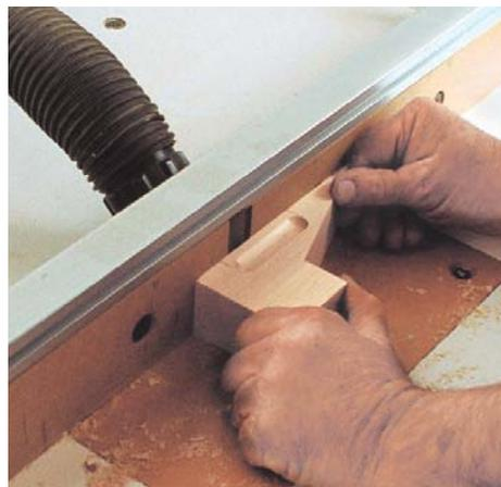
**Rout the finger groove.** A shallow finger groove on each side of the plane is cut on the router table using a cove bit.
