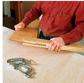
**A testing square is used to square up the jig.** A long blade and notched handle make up the testing square. When the two parts are clamped together, the glue-up jig is ready to be squared.
