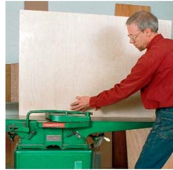
**For the jig to be accurate, the base must have a perfectly straight bottom edge.** A good factory edge works fine, but if you have doubts about the straightness of the edge, run it over the jointer a couple of times.
