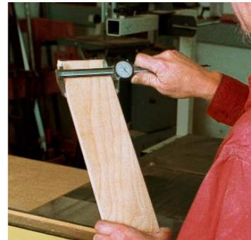
**Check the reference board for parallel.** The width of the reference board should be the same within a few thousandths of an inch along the board's length. If you have a caliper, this is a good time to use it.
