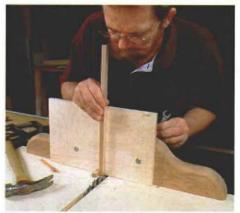
Adjust the jig. To find a starting point, use the leftover length of spacer material to locate the spacer block ½ in. to the right of the dado blade, then tighten down the bolts.
