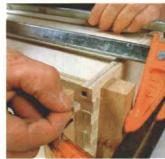
Fill the void. The groove for the top and bottom can be filled easily with end-grain plugs of plywood. Once glued in place, you'll have a hard time spotting the fix.
