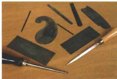
Scrapers come in many sizes and shapes. Aside from the standard card and gooseneck shapes, you can grind custom profiles to fit everything from beads to coves and use thin scrapers to wrap around curves.
