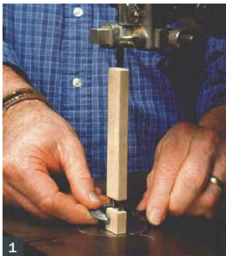
1 Relax the blade tension. Then clamp the short block of the gauge to the side of the blade, just behind the teeth.
