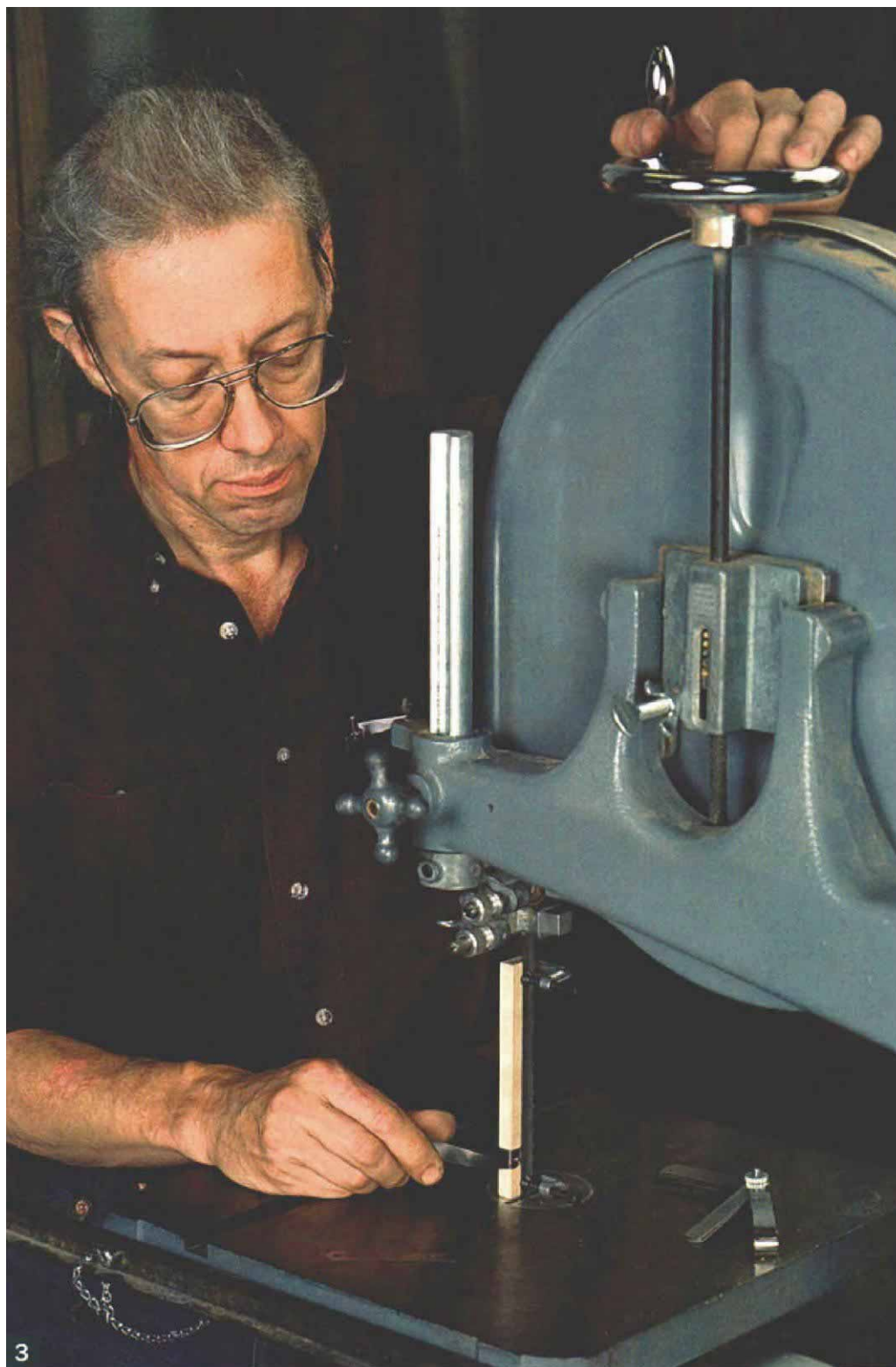
2 Leave room for the feeler gauge. Clamp the long block to the blade so that a 0.005-in. feeler gauge fits between the block and the measuring pin.
