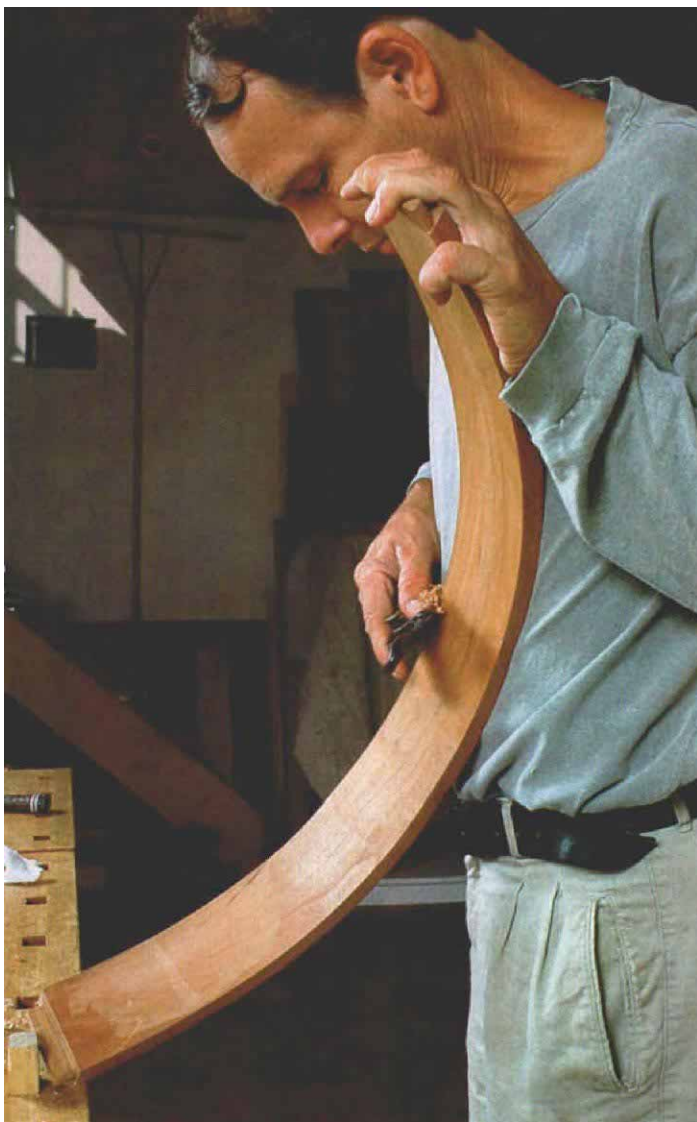
Spokeshaves are good for concave curves. Lightweight enough to use with one hand, this Stanley No. 54 has an adjustable mouth to help control the depth of the cut.
