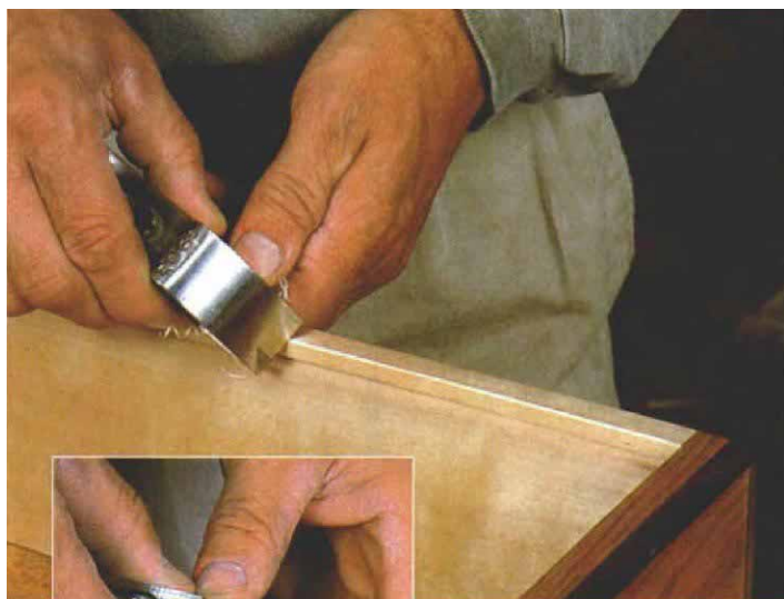
Use the Stanley No. 90 bullnose plane for cutting inside chamfers. Start inside chamfers with a few quick cuts, then cut close to the corner. Pare away the remaining wood by using the tool as a chisel plane.
