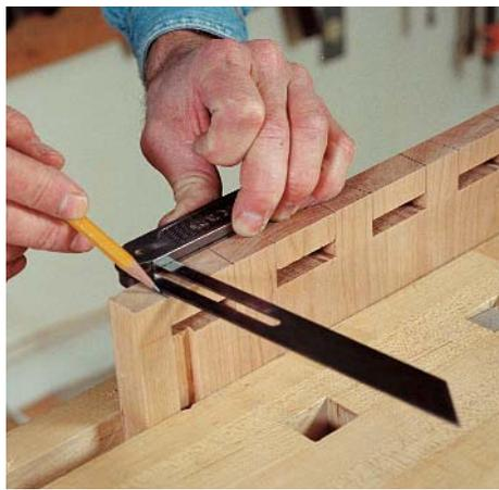
**Mark the tapers for the mortises.** Use a bevel gauge set for 6° and mark the edge, then transfer the marks to the bottom face with a square.
