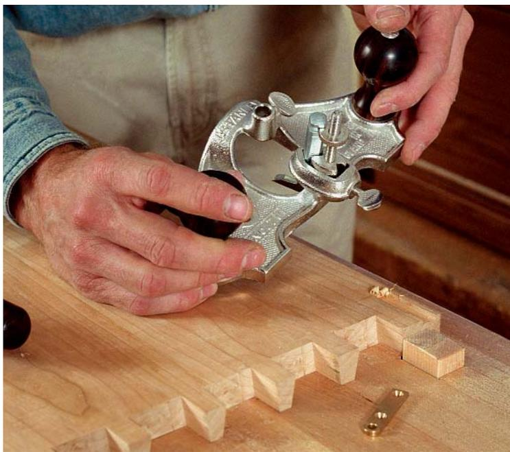
**Rout knife-hinge mortises in the case.** It's much easier to cut mortises before gluing up the carcass. The author used a router plane.
