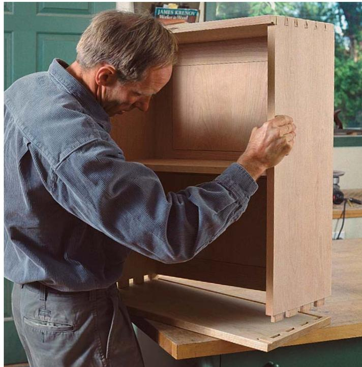
**In the first glue-up, the sides are joined to the top, back and shelf.** It's less stressful to leave the bottom for last and not have to worry about trying to get everything done at once before the glue sets.
