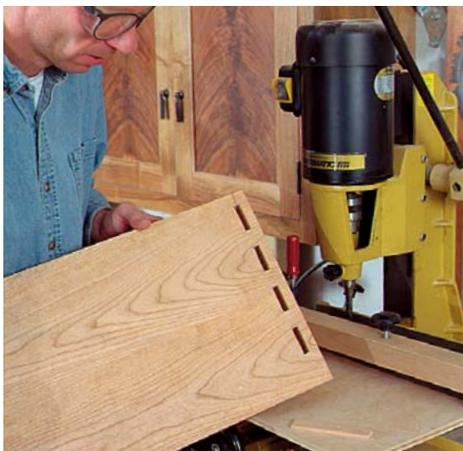
**Cut through-mortises.** Cut halfway through one side, then flip the stock and finish from the other side to avoid tearout.
