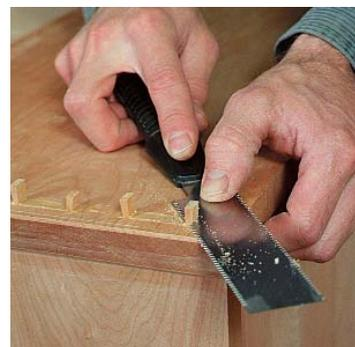
**Spread glue on the surfaces of the mortises, tenons and wedges.** Gently tap the wedges in place. Clamps hold the carcass together. After the glue dries, trim the wedges. A flush-cutting saw makes the job easier.
