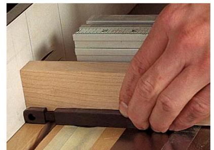
**Cut 3/16-in. square tenons on the posts.** Each blank is good for two posts, one on each end.
