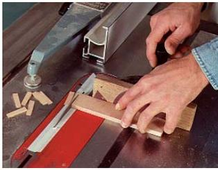
Wedges are driven into slotted tenons that fit into tapered mortises. In cross section, this joint resembles a dovetail. When making the wedges (left), set the miter gauge on the tablesaw to 3°, cut one side, then flip the stock and rip off a wedge.
