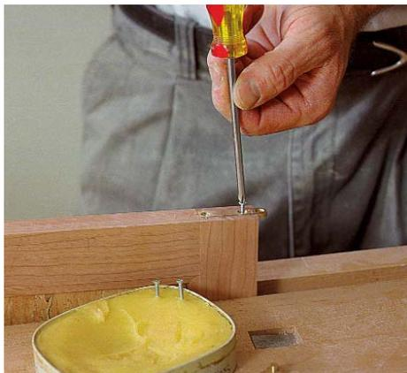
**Mortise the doors and attach the knife hinges.** Note that the pivot pin must be located beyond the door's edge. Use waxed steel screws to cut the wood fibers. Later, replace them with the delicate brass screws.
