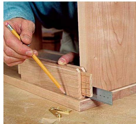
**You need a slight gap between the door and edge of case.** The author uses a 1/16-in.-thick ruler as a shim, then transfers the location of the knife hinges.
