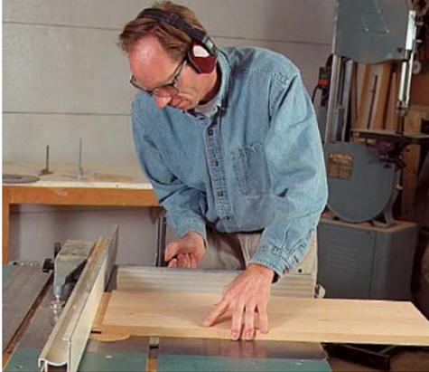
**Machine one long tenon on each side of the case.** The author cuts the tenons slightly deeper than the mortises; the excess will be trimmed off after the glue-up.
