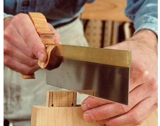
**Cut slots in the tenons.** Each tenon receives two slots. When wedges are driven, the tenons flare out, creating a secure joint.
