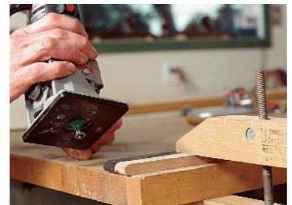
**Begin with an ebony blank 3/4 in. thick by 3/4 in. wide and 12 in. long.** Rout the ends with a 1/4-in. radius roundover bit. The adjoining piece prevents tearout.
