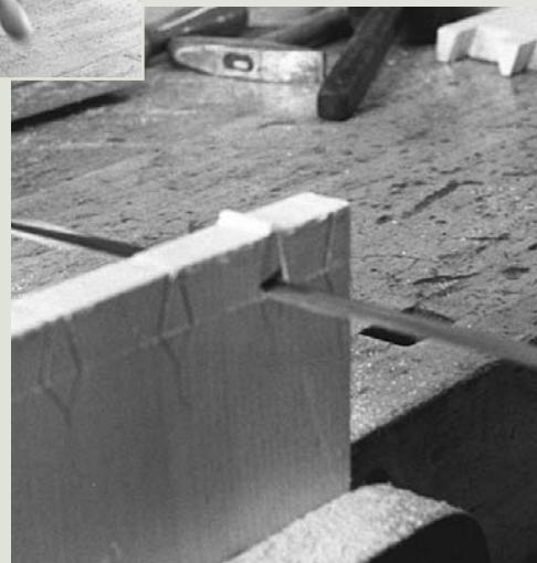
**How it cuts.** The front of the blade cuts vertically. Then, as the middle of the blade is engaged, the saw begins to turn the corner and cut the bottom of the socket. The bottom cut is finished using the horizontal back end of the blade.
