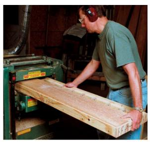
The entire sled goes through the planer. Multiple passes will probably be necessary to produce a flat side.
