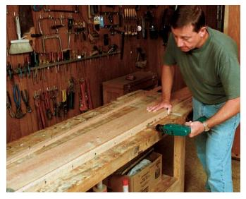
The leveling-strips method for twisted lumber. The plank is placed on a flat surface, and shims are placed under the high corners to even them out. Hardwood strips (¾ in. thick) are then screwed onto the sides, using 1¼-in. multipurpose screws. The strips offer three possible hole positions at each location.
