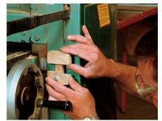
A small go/no-go gauge identifies boards that fall within the planer's <sup>1</sup>/<sub>4</sub>-in. cut. Many sawmills don't deliver boards of uniform thickness. Valuable time is wasted when a tapered board binds in the planer or a thin board won't feed. Too-thick and toothin boards are put aside for later passes.
