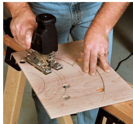
Cut out the opening. To achieve a nice radius, drill \frac{3}{4} -in.-dia. holes in the corners before cutting out the opening with a sabersaw.
