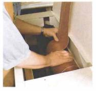
Access is good inside the Woodmaster, and that makes abrasive-strip changes easy. A hook-and-loop system keeps the strip in place.
