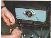
By turning a pair of jackscrews, Delta's table may be realigned to the drum.
