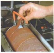
Performax supplies a special tool to hold the clip in place while the abrasive strip is installed. The Delta doesn't need a tool; the Ryobi could use one.
