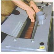
The RBI has less working room under the hood. Hook and-loop abrasive strips are also used.
