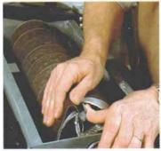
Cantilevered machines use clips to hold the spiral-wound abrasive strip in place. One end of the drum has a clip under spring tension to take up slack should the abrasive strip stretch.
