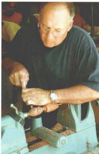
Flame on. George Slack carves a flame finial, using the lathe as a vise.
