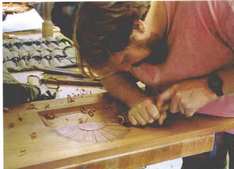
Shaving the shell. Bob Smith works on the center shell on the lid of his secretary.
