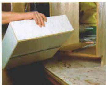
Locate the slide along the centerlines of the cabinet divider and the drawer. The slide screws into the drawer bottom, so use material that's at least \frac{5}{8} in. thick.
