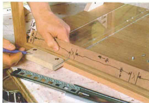
Mark the location of drawers and slides on a story stick. Used in tandem with a jig, the story stick ensures accurate placement of the slides inside the cabinet.
