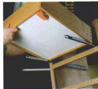
The drawer sits on top of the runners. Notches are cut in the back to clear the runners.
