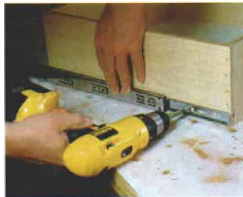
Ball-bearing slides are installed flush with the bottom edge of the drawer sides. Use a flat surface such as a workbench when installing them.
