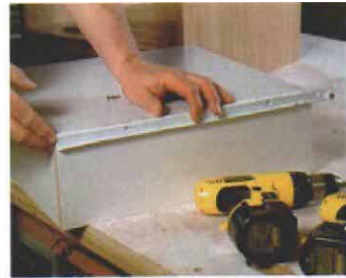
Roller slides are easy to position. The L-shaped runners wrap around the undersides of drawers.
