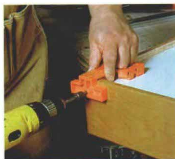
The rear of the drawer is bored out using a jig, too. The holes are for hooks located at the tail ends of the runners.
