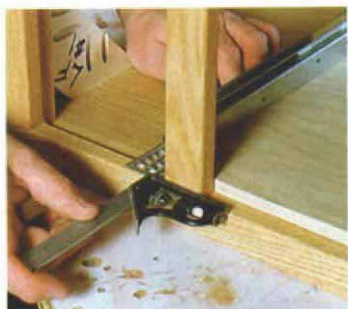
Use a piece of scrap plywood to position the slides inside the case. Also, set the slides back from the edge of the case, as per the manufacturer's instructions.
