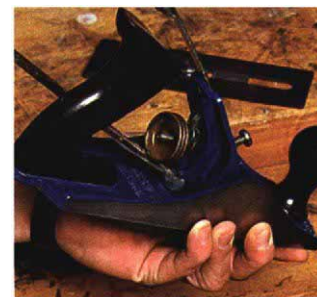
Adjusting the frog. To get an especially thin shaving, loosen the screws on the plane's frog and move it forward, adjusting until the blade has only the slightest opening.
