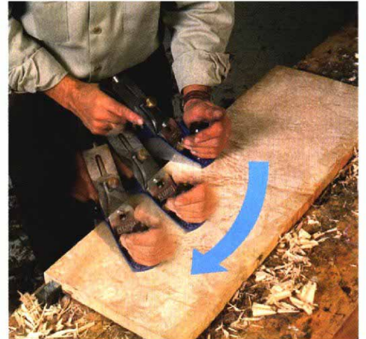
A sweeping cut. For difficult figure, such as bird's eye, set the blade for a thin cut and take skewed, arching passes.
