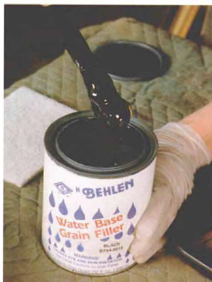
Stirred, not shaken. Water-based filler should have the consistency of thick latex paint.
