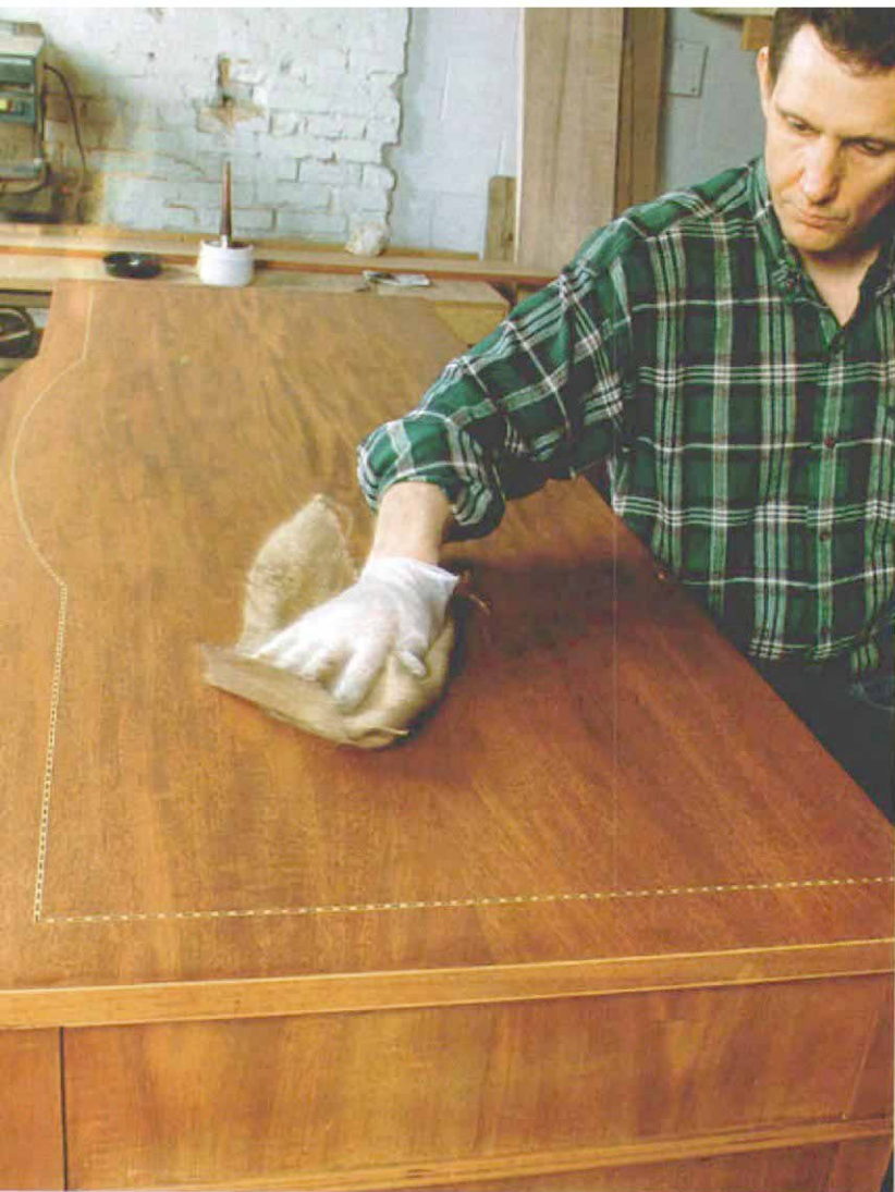
Use burlap for a final wipe. A quick, vigorous rubdown will remove marks left by the squeegee and any traces of excess filler remaining on the surface of the wood.
