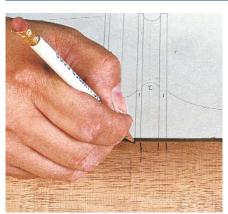
This step is worth every minute. Taking the set-up time to mark the turning lines prominently on the blank will help you avoid costly mistakes.
