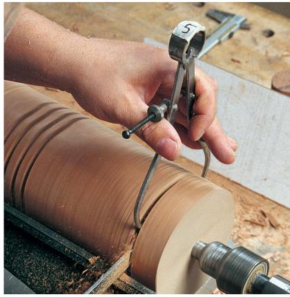
**Make it simple with a system of numbers.** The author codes his calipers to correspond to different finished diameters on the workpiece.
