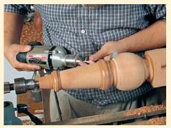
**Hand drill as power sander.** The author uses quick-change sanding discs in the final stages of shaping each leg.
