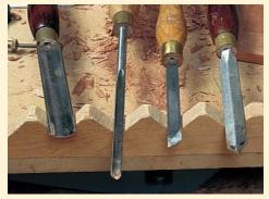
You don't need a wall-full of tools. Gouges, a skew and a parting tool were the only turning tools used to make the legs for this article.
