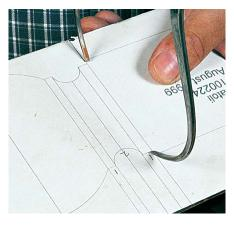
A pattern is a map and a story stick. You can use a full-sized drawing of the workpiece to set calipers and to monitor your progress after you start turning.
