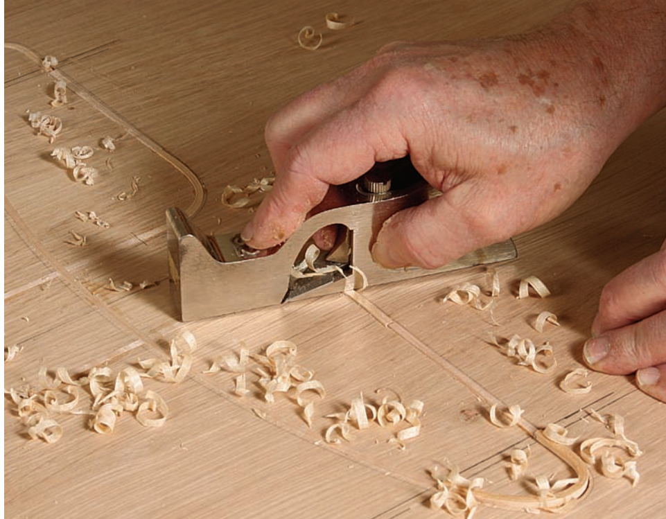
Add the last sections. Cut and fit the rest of the string inlay, then flush the entire pattern to the panel.
