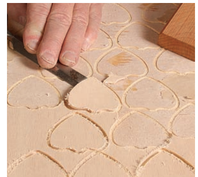
Rout out and free the shapes. Use a 1/4-in.-thick Masonite template and a 1/8-in. straight bit and bushing to cut each shape (above). Then use a chisel to pop the shapes off of the backer board (right).
