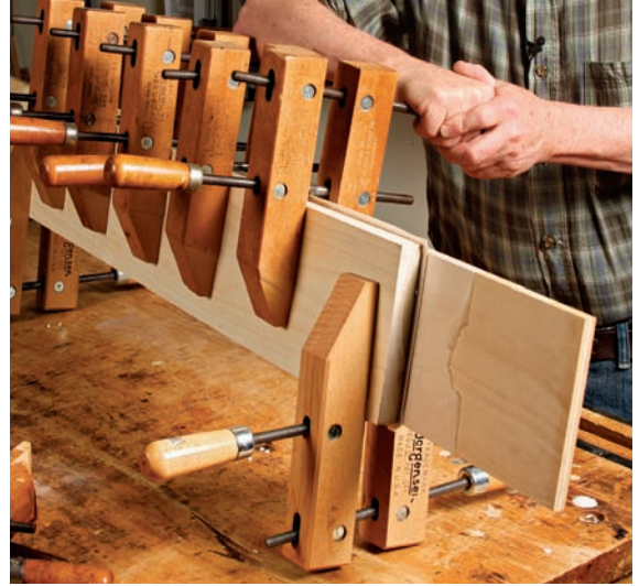
Glue the veneers to a backer. For the spades and heart inlay, Rodel glued the veneers to a backer board first, with the veneer separated by newsprint.
