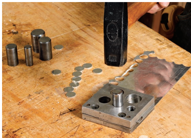
Punch out the centers. In the center of the spade and heart inlay, Rodel inserts a 5/8-in.-dia. metal disk. He uses a special punch to make the disks ( jewelrysupply.com ).
