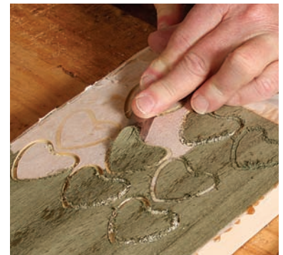
Glue the veneers to a backer. For the spades and heart inlay, Rodel glued the veneers to a backer board first, with the veneer separated by newsprint.
