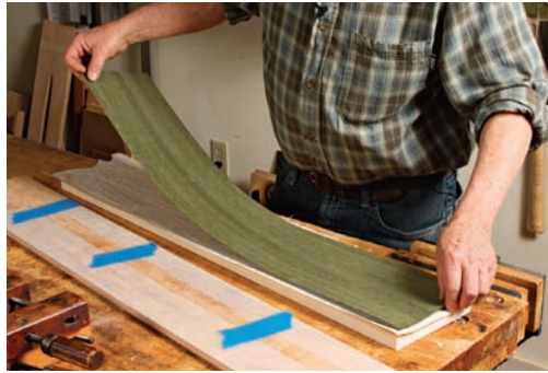
Glue the veneers to a backer. For the spades and heart inlay, Rodel glued the veneers to a backer board first, with the veneer separated by newsprint.
