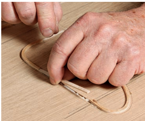
Add the last sections. Cut and fit the rest of the string inlay, then flush the entire pattern to the panel.
