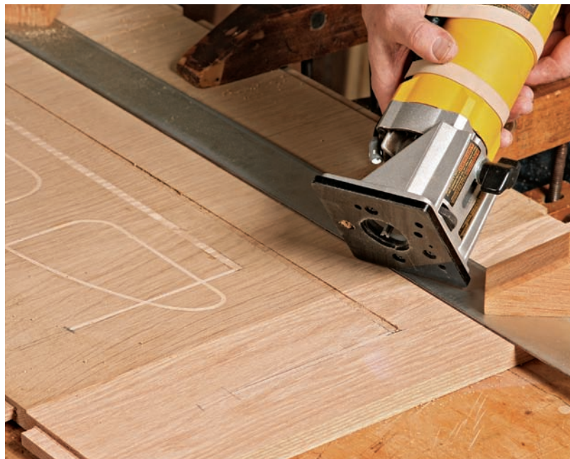
Wide sections are next. Use a router with a straightedge to cut the channels for the 1/4-in.-wide sections of inlay. Then glue in those pieces.
