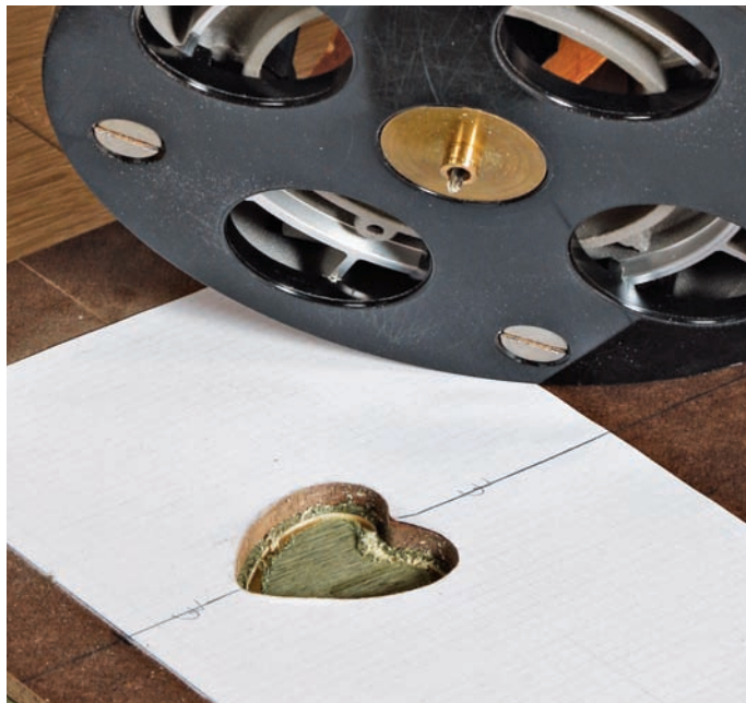
Rout out and free the shapes. Use a 1/4-in.-thick Masonite template and a 1/8-in. straight bit and bushing to cut each shape (above). Then use a chisel to pop the shapes off of the backer board (right).
