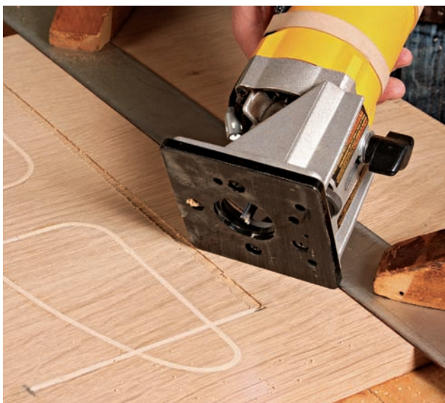
Wide sections are next. Use a router with a straightedge to cut the channels for the 1/4-in.-wide sections of inlay. Then glue in those pieces.
