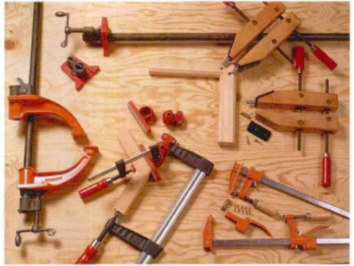
Accessories can improve your clamping range. Clockwise from left: Mastodon's Jaw Extenders; Brink & Cotton's Stand-Up pads, hand-screw adapter tips that fit pocket holes to tighten joints; E-ZHold adapters that add a trigger to a Jorgensen bar clamp; and Bessey's Irregular-Angle set for clamping at odd angles.
