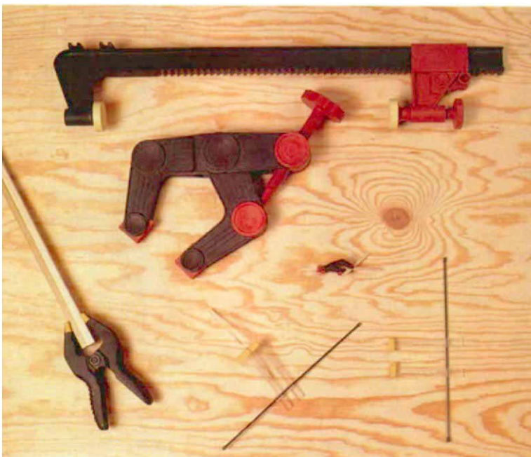
Plastic clamps suit delicate jobs. The rubber pads of Quick-Grip's spring clamp (left) are gentle on work. BTM's lightweight polymer clamps (top) resist rust and solvents. Their miniclamp and Testfabric's clear acrylic clamp are good for restorations.
