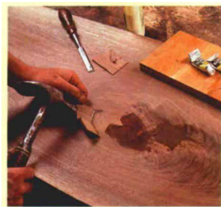
Step A: Filling the knot involves spreading a mix of epoxy and sawdust into the cracks and then driving and gluing in shaped wedges into the gaps.
