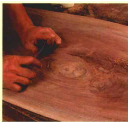
Step B: Smoothing the surface with a scraper blade at various angles all around the knot and its reaction wood shows that the surface is now solid.
