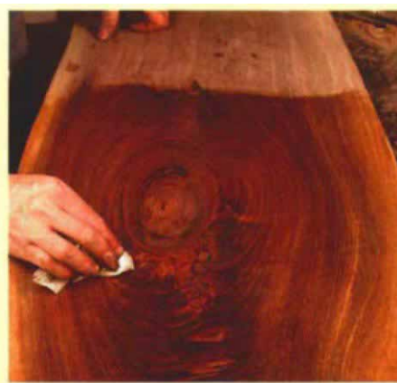
Step C: Oiling the wood reveals the colors of the repaired areas. Darkening the fillers with dye will finish them to a near perfect match of the knot.
