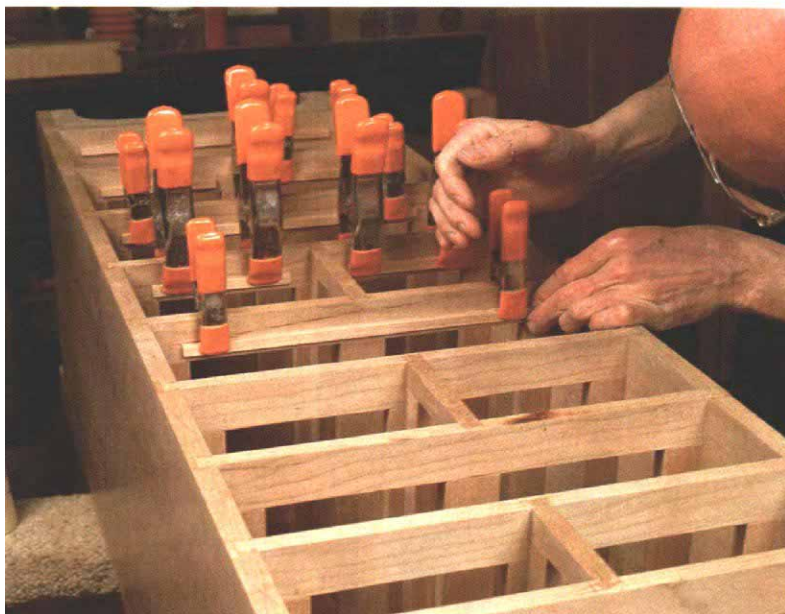
The drawer stops are glued, positioned on the dividers and held in place with spring clamps. The stops must be thin enough to clear the drawer bottoms and short enough to allow drawer side clearance at the ends. Leather bumpers are temporarily glued to the stops to position the drawers for sanding.
