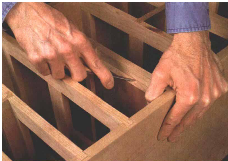
Scribed lines accurately position stops —The author uses a 4-in.- to 6-in.-wide board, cut to the appropriate length, as a gauge to scribe alignment marks for the drawer stops. Measuring from the cabinet back eliminates any variations that may have occurred when gluing in the dovetailed drawer dividers.
