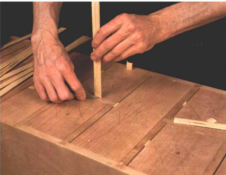
Wedging the drawers in place holds them for beltsanding. The drawers should be wedged on each side to center them in the opening and wedged at the top to hold them firmly against the drawer dividers and stops. The entire front of the cabinet can then be sanded to one flat, smooth plane.
