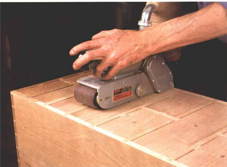
Sanding the cabinet front, with the drawers held in place by front-mounted stops and wedges, ensures that the entire face of the cabinet will be flat and smooth. The drawers support the sander and prevent gouging the face frame. This technique eliminates the need to set each drawer individually.
