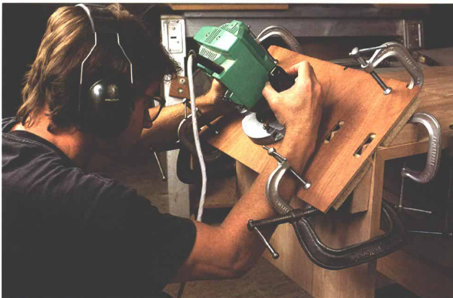
Keyed miters —Two sides of an alder toy box (above) show how attractive a keyed miter joint can be. To rout key grooves in big mitered carcasses (left), it's safer with a simple jig.
