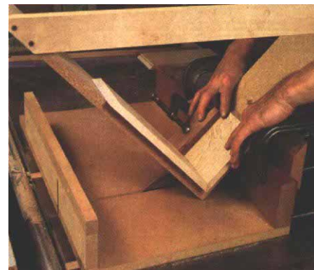
The author's jig for cutting grooves for keys clamps right into his crosscut box. For boxes that fit safely into this jig, three keys provide plenty of strength.
