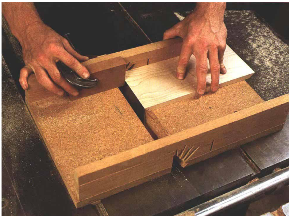
Cutting the groove for a spline in a miter joint is simple using a clamped stop block in a sliding crosscut jig. The stop block ensures that the groove for the spline is positioned in the same place in both boards being glued together.
