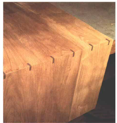
Keyed miters —Two sides of an alder toy box (above) show how attractive a keyed miter joint can be. To rout key grooves in big mitered carcasses (left), it's safer with a simple jig.
