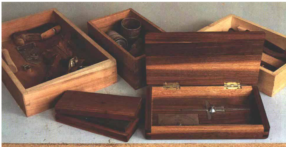
Choosing an appropriate joint for a box is as much a matter of personal taste as it is an engineering decision. Boxes in the author's shop include a drawer featuring, through- and half-blind dovetails, a simple rabbeted plywood box and three-finger-jointed boxes.
