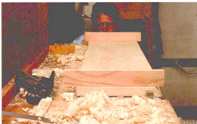
Sighting along winding sticks tells the author that the board doesn't twist. He also uses a long straightedge to check flatness along and across the board's length.
