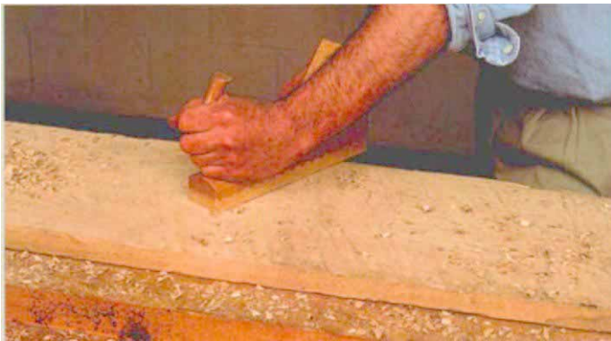
A scrub plane makes quick work of high spots on the rough board. Korn planes across the grain diagonally to prevent tearout and then planes on the opposing diagonal, removing the ridges created with the first passes. A bench plane is the next step.
