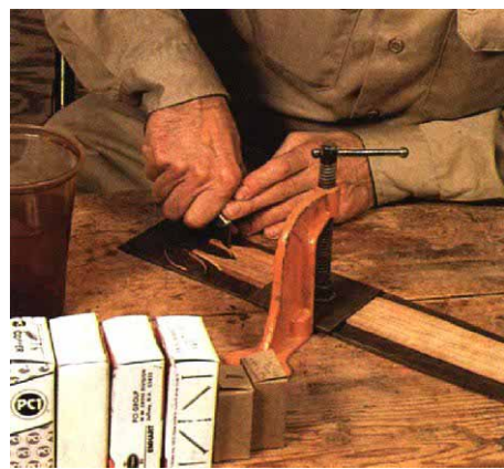
Beveling the finger edges and ends is much easier if the band is first soaked in hot water and securely clamped to the bench. Reposition the hardboard cutting block for each finger set so that knife kerfs from previous cuts don't affect the cut.
