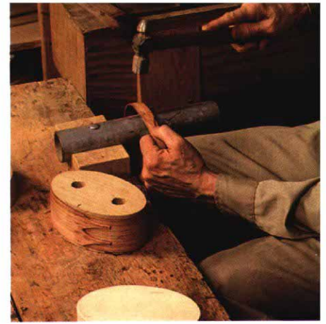
Tacking bands with an anvil backup, clinches the tack. Once tacked, the top band will be dried in place on the box band. Shapers in the box band on the bench keep the band's oval shape while it dries.
