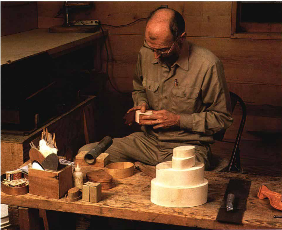
Tacking bands with an anvil backup, clinches the tack. Once tacked, the top band will be dried in place on the box band. Shapers in the box band on the bench keep the band's oval shape while it dries.
