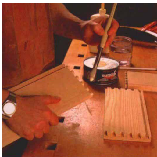
Use a stiff brush to work glue down into the pins. Don't apply glue in the sockets because it can pool up and keep the joint from closing.
