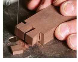
Cut the tails. After establishing the shoulders, Latta cuts the tails on the scrollsaw, getting close to the layout lines, and then pares them clean with a chisel.
