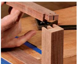
Transfer the tails to the top of the leg. Registering on the shoulder, score the ends of the tails on the top of the leg (above). For a tight fit, mark one side of the tails, move the board to just cover those lines, and then mark the other side. Rout the pin sockets, pare them with a chisel, and test the fit (left).
