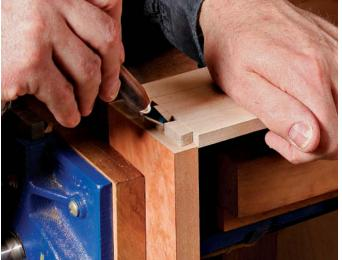
Cut the tails, create the shoulder, and mark the drawer front. Set a marking gauge to the thickness of the tails and score the drawer front. Then, registering on the shouldered tails, transfer them to the drawer front with a knife.
