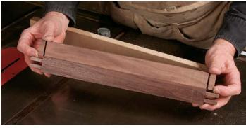
**Creating the** shoulder. Latta uses a miter gauge on the tablesaw to make the shoulder cuts on the faces and edges of the tail board. Using a test piece, creep up on the shoulder-toshoulder distance until the shoulders exactly match those of the lower stretcher to ensure a square opening (above). Then, use a tenoning jig to make the cheek cut on each end of the upper rail (right).
