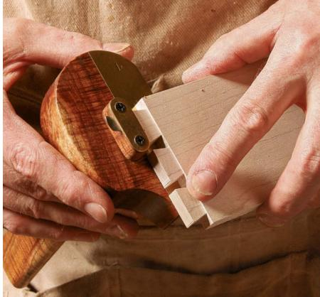
While creating the shoulder on a dovetailed drawer makes a huge difference to the stability and appearance of the finished product, shouldered dovetails aren't much more work to create.
