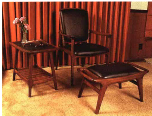
Angled tenons—some compound—were used almost exclusively in the construction of this walnut chair, stool and side table. Legs on two of these pieces splay in two directions, requiring slightly angled tenons at both ends of apron pieces, stretchers and seat supports.
