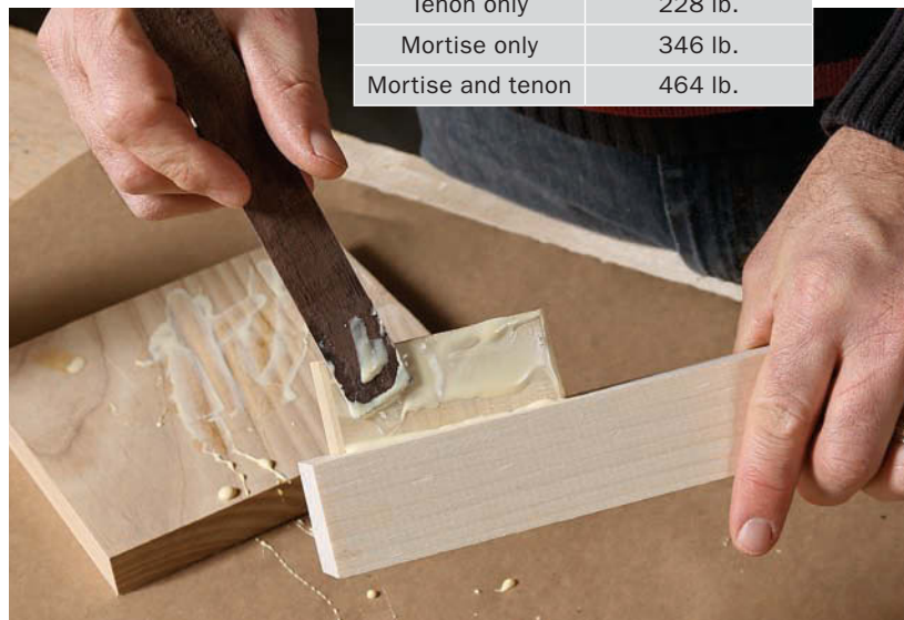
All tenons were \frac{3}{8} in. thick by 2\frac{1}{4} in. wide by 1\frac{1}{4} in. long.
