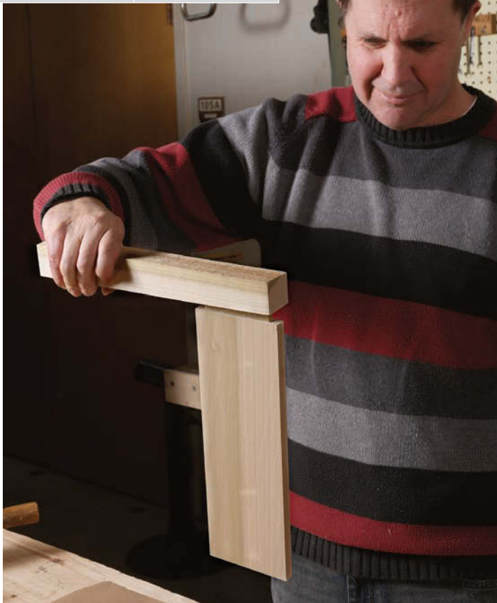
All tenons were \frac{3}{8} in. thick by 2\frac{1}{4} in. wide by 1\frac{1}{4} in. long.
