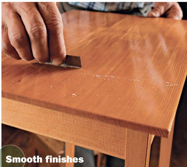
**They work for finishes, too.** Hack uses wider square-edge scrapers to remove dust nibs and other imperfections from tabletop finishes. A well-honed scraper will leave a glasslike surface.
