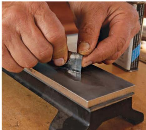
**Hone and polish.** Hack hones the edges of the scraper on a fine diamond plate and a 2,000-grit waterstone. He polishes the faces first on a 2,000-grit waterstone and finishes with 5,000-grit. He polishes only the area near the cutting edge. For these cleanup tools, a burr is not necessary.
