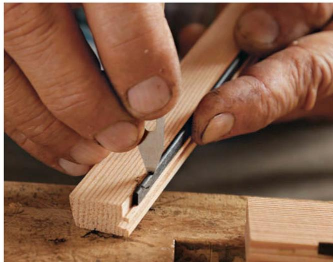
**Beadwork.** This ebony bead is smoothed with a narrow scraper with a hollow nose that matches the bead profile. A light touch creates delicate shavings.
