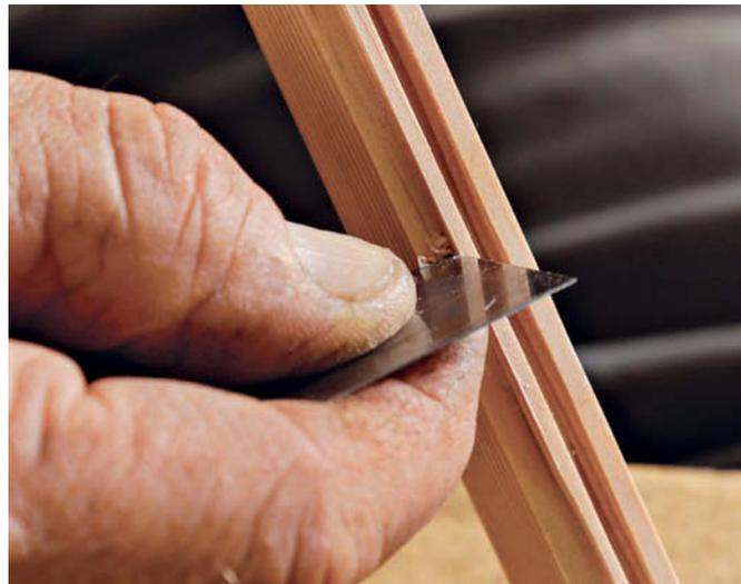
**Coves and fillets.** This curly maple molding had some tearout. To clean it up without losing detail, Hack uses a rounded scraper for the concave section (left), and a square scraper to finish the fillet (above).
