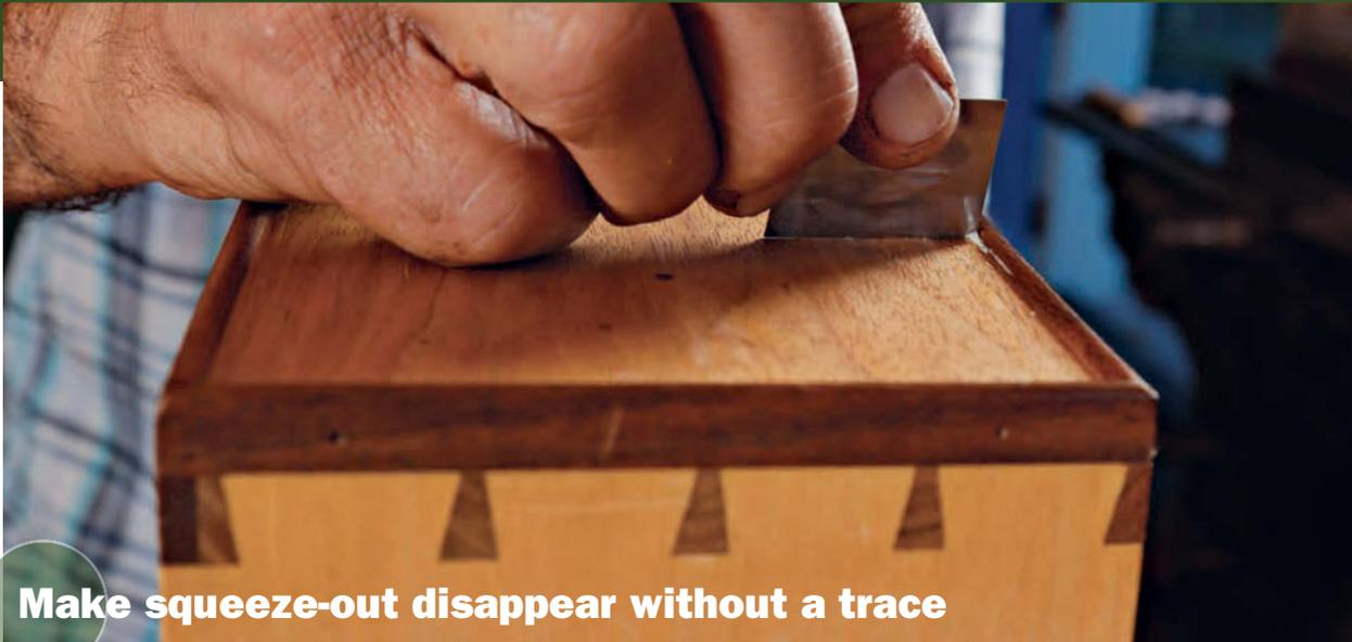
**Clean up the cock bead.** For this delicate job, Hack uses the straight-edge scraper to get the glue out. Again, the vertical edge of the scraper has a slight angle so it can reach into the corner without damaging the applied bead.
