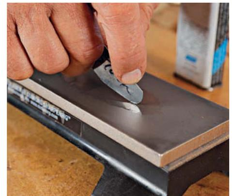
**Trace the profile.** After cutting the blank to size, use a fine Sharpie to trace the profile on it (left). Shape the profile with a file, then hone the edge and polish the faces in the same way you'd work a square-edge scraper (above). For hollows, you'll need a chainsaw file or jeweler's files to create the profile. Don't use a grinder with this thin steel, as it will ruin the temper.
