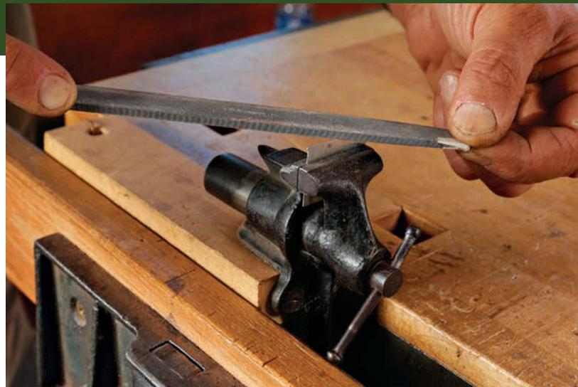
**Snip and file.** Hack cuts small scrapers from an old Japanese handsaw blade (left). More robust scrapers are taken from thicker western saws. For a straight scraper, he snips it out of the blank, then cleans up the cuts with a file (above), holding the blank in a small vise.
